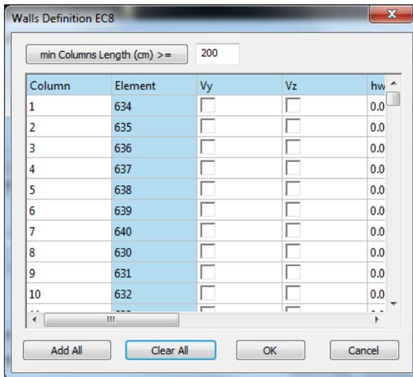
Enter the min Length (cm) and select the "min Column Length" command to automatically define the walls per direction. The program automatically calculates the sizes required to calculate the eigenperiod.
