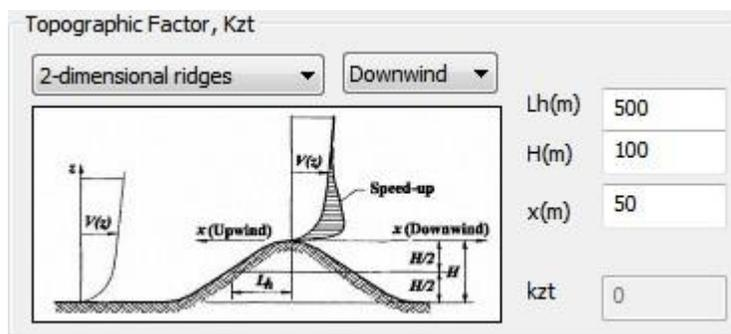
refers to the influence of the topographic configuration of the area in which the structure is located (FIGURE 6.4-2). The parameters are selected on the basis of which the Topographic Factor (Kzt) is calculated.
