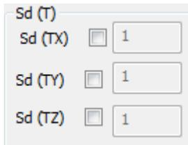
activate the coefficient for the corresponding spectrum and enter the value. For example, if you set  $Sd(TX)=2$ , the values of the design spectrum in the X direction will be doubled.
