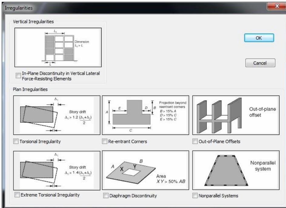
the planner determines in the Plan Irregularities section whether the corresponding criteria are met by checking the reverse option.
