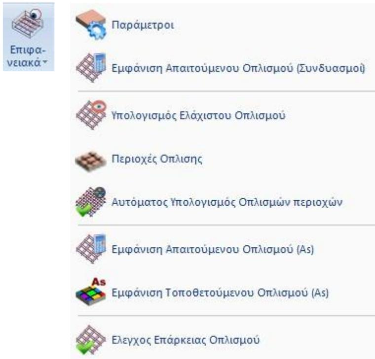
In the new version of SCADA Pro a new integrated tool has been added for calculation and design of reinforcement of foundation or superstructure slabs, slabs which have been simulated with surface finite elements.
