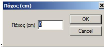
Select the command and in the dialog box:
