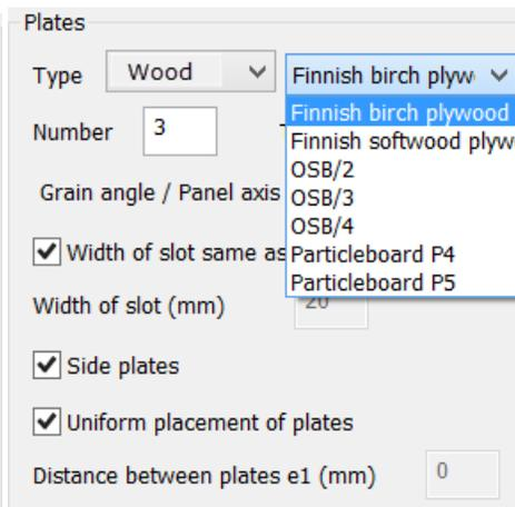
⚠ In case of **Wooden Flange**, the parameter **Grain angle / Panel axis** where the user defines the angle of the grain of the wooden flange as to the axis of the Main member, is activated.
