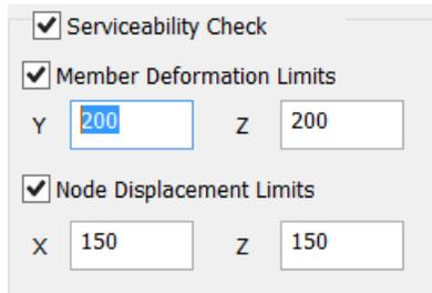
Then type the corresponding values in each direction, X, and Z. For example in the figure on the left, the limits are defined as  $l/200$  and  $l/150$ , where  $l$  is the member’s length.
