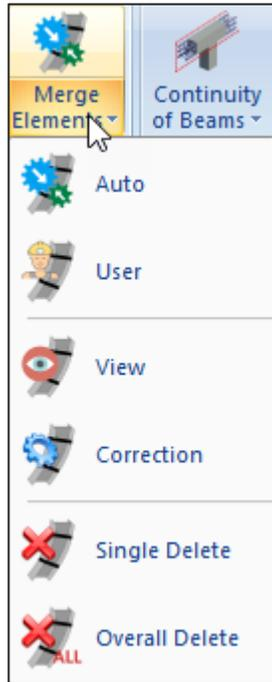
Merge elements mean that the individual parts of a single element, merge in each buckling direction, either automatically or manually.
