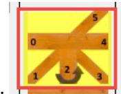
**Direction:** The direction of each member is defined according to the icon. Therefore, start by selecting the left-hand member to define the 0 directions and continue defining the direction of the remaining members of the connection.
