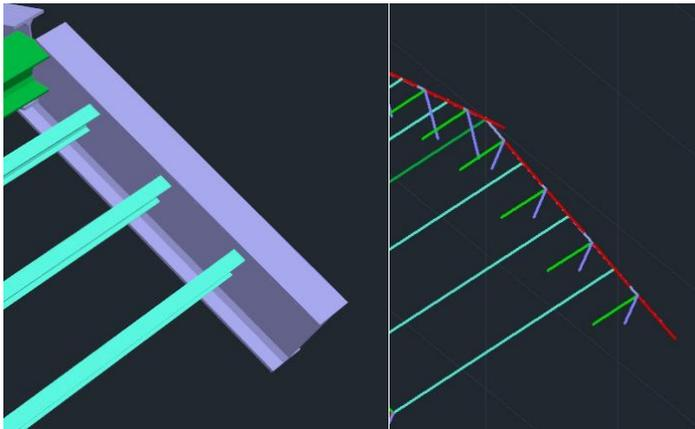
The local axis of the beam that is parallel to the purlins is the y-y. So,  $L_y$  will be the merged length of the total beam, while  $L_z$  will be the single members.
