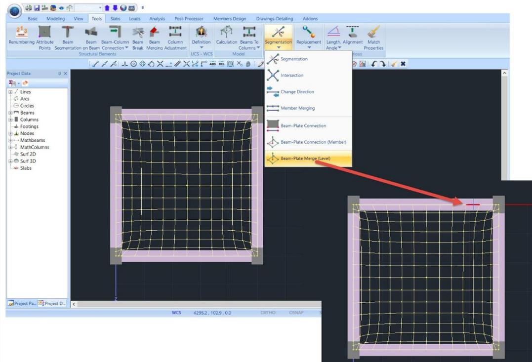
Consequently, by breaking the beam in small parts, the need for merging is born, for the beam to be designed as a single member. This is accomplished by using the command Merge Beams.
