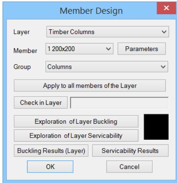
A check is performed by layer. So first select the layer from the drop down list and the "Member" list shows all members of this layer and its cross sections.
