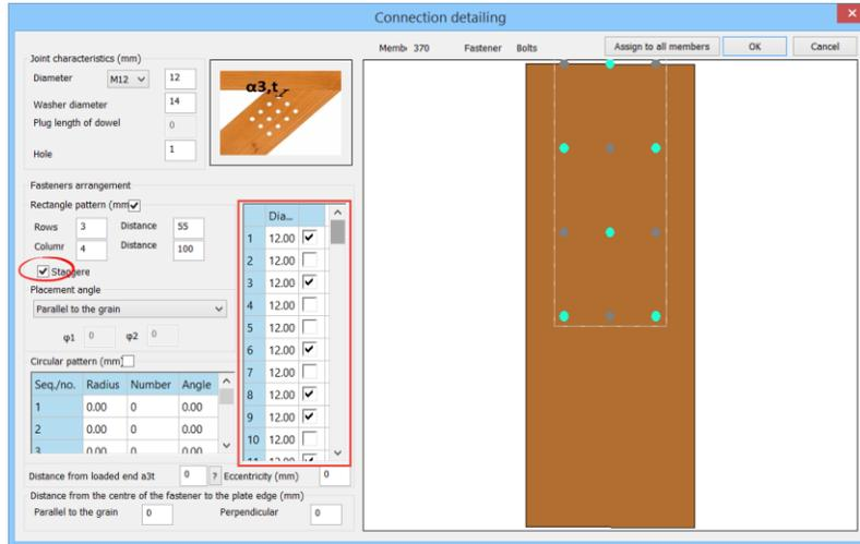
The **Placement angle** of the connectors is selected from the list and is displayed in the figure.
