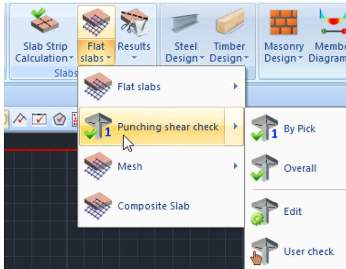
The punching checks are also added in the new version by EC2. The check is part of the check and design process of the flat slabs which runs automatically, but can also run as an individual check for any column. All data can be set automatically or even manually.
