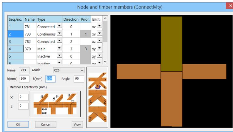
**Angle:** Is the angle of the member as to the connection. The angles are defined counterclockwise with 0 in + x.
