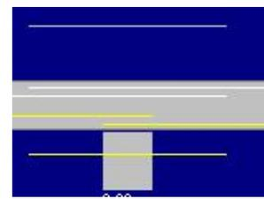
On the common support, the positioned bars consist of two different bars. By clicking on the two bars, they are converted into one common bar.
