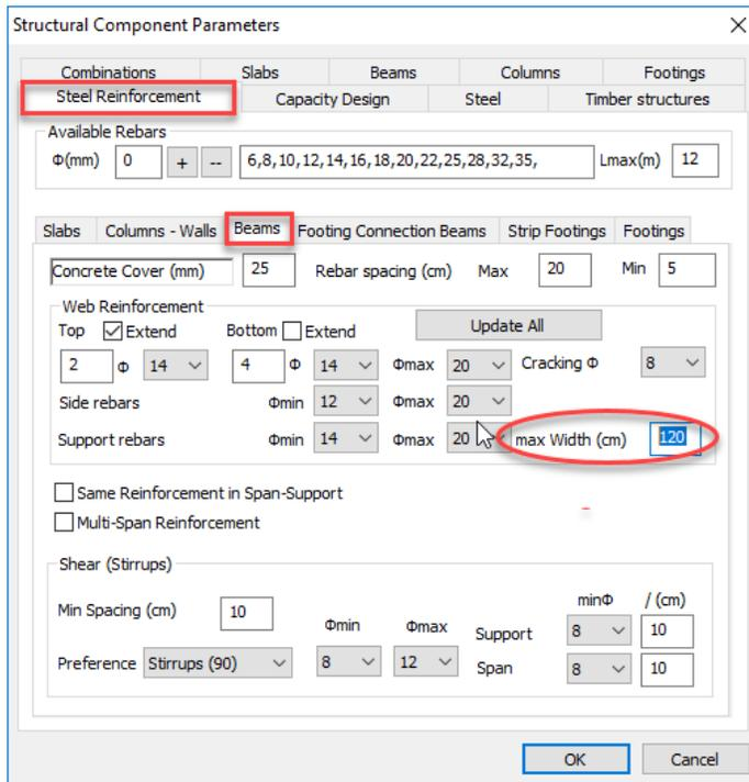
If it exceeds the max support width (see Figure 1), then support reinforcement per side is placed separately.
