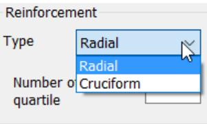
Finally, in Reinforcement set the layout type of punching reinforcement choosing between Radial and Cruciform. For the Radial layout set the number of radii per quartile.
