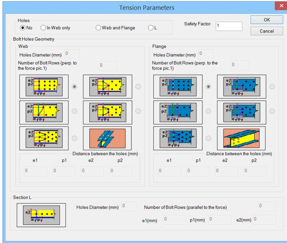
Specify the spacing of the centers of two consecutive holes, the holes diameter and the number of bolt rows.
