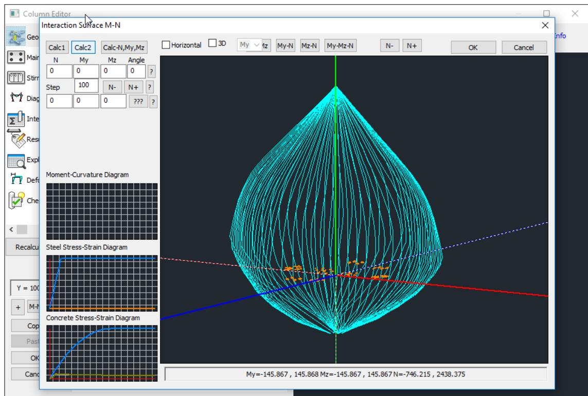
⚠ The calculation of the interaction diagram M-N can also be performed for a single column or wall, using the command “[Detailing](#)” (see the corresponding [chapter B. Column’s Detailing](#)).
