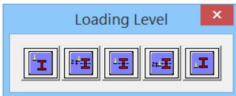
Determination of the Loading level of the member. The following five options are displayed by selecting the icon.
