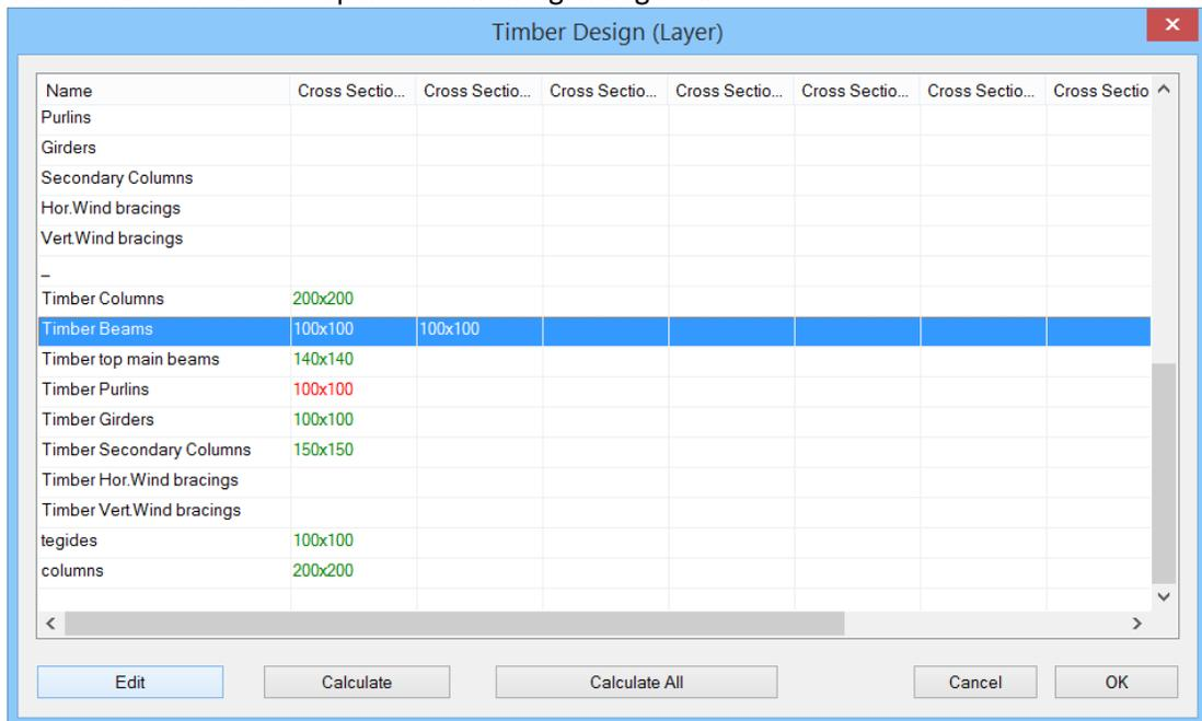
The first column contains the layers of the current project and the other columns the cross-sections that belong to each layer.
