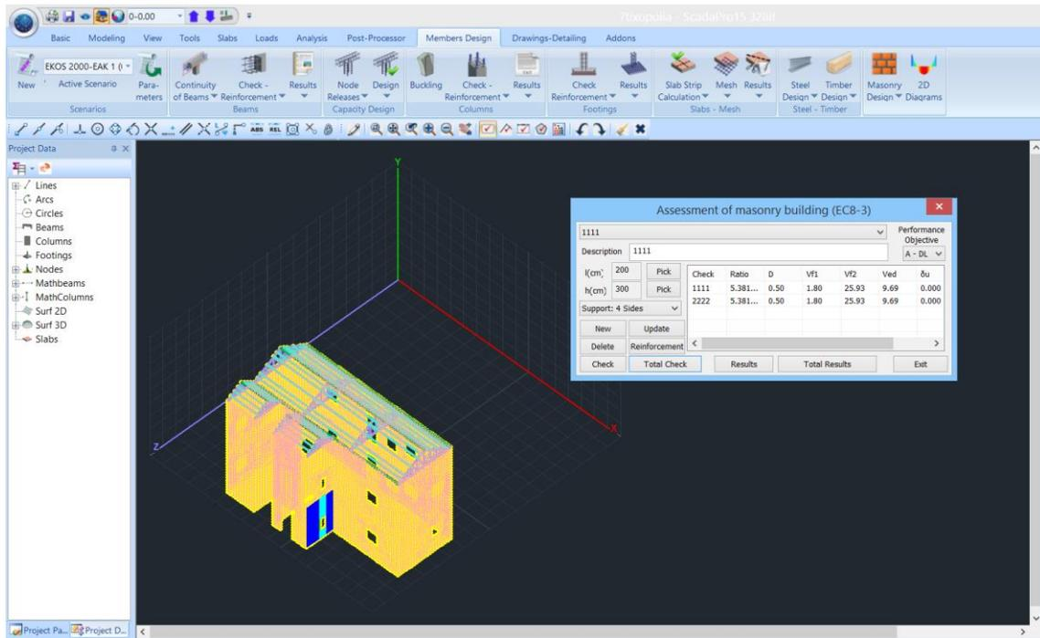
⚠ The adequacy checks are performed per pier/spandrel section regarding forces and deformations depending on the Performance Level.
