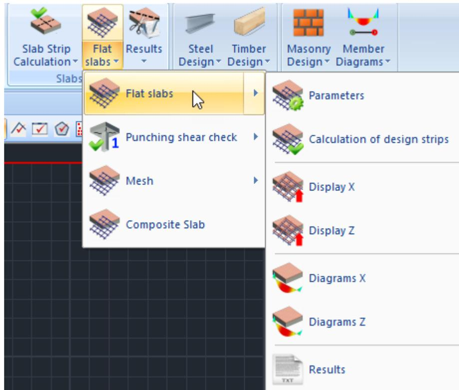
The new version of SCADA Pro offers the possibility of creating flat slabs (slabs without the presence of beams) with the finite element method.
