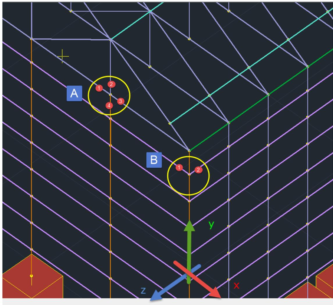
The connection A is in XY level i.e. the steel connecting plate will be introduced at this level (vertically).
