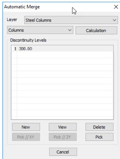
Considering that, the columns merging will be interrupted at 300.00 cm. The column will merge from 0.00 to 300.00 cm and the next floor column from 300.00 to 600.00 cm.
