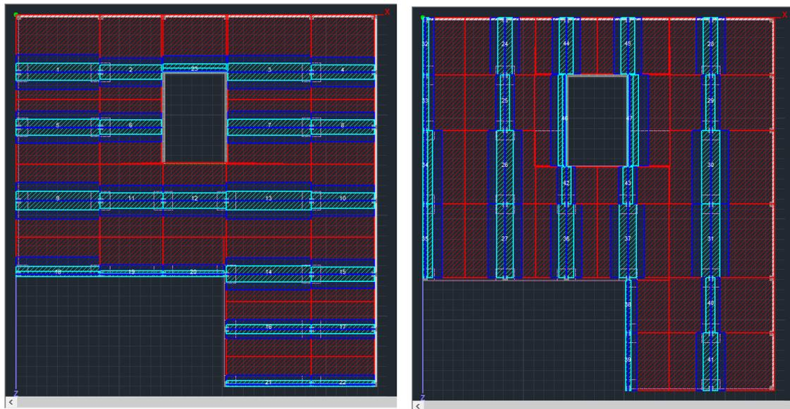
Design Strips along the X and Z axes
