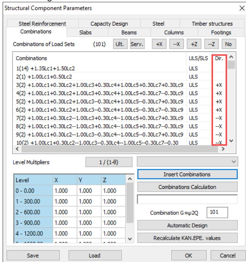
A combination is defined per x or z if the corresponding seismic force has a unit coefficient.
