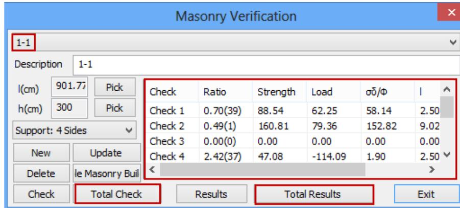
The design checks are applied to sections (horizontal and vertical) concerning the EC6 design code.
