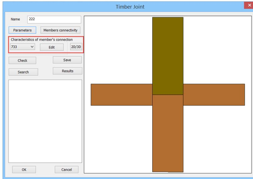
After Member’s connectivity and Parameters definition, the connection’s **Editing** follows. Choose a member, starting from the *Main*, either graphically in the right figure, or from the list
