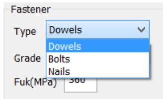
In the **Fastener** field define the connector **Type** (between Dowels, Bolts, and Nails) and the **Grade** and the **Fuk** tensile strength value is automatically updated.
