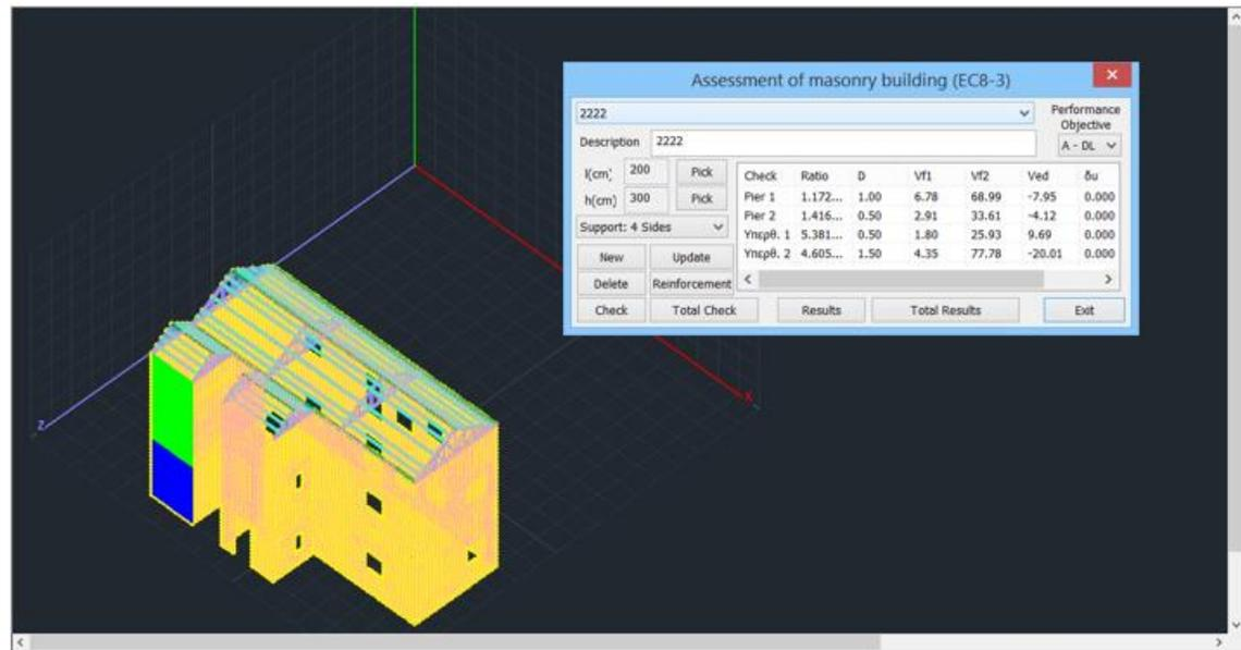
**Total Check** to make all the checks for all the defined walls and each pier/spandrel section.
