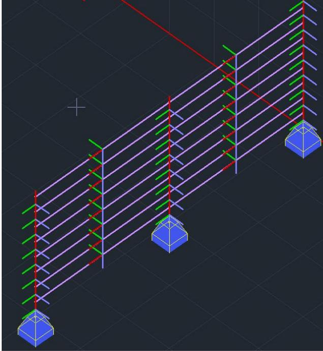
The supports from the columns are parallel to the local z-z axis (blue, out of plane) of the griders. So, merging will be in  $L_z$  (total length). While in the y-y direction (green, in the plate),  $L_y$  is the length of each member.
