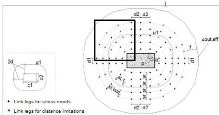
Radial reinforcement Layout
