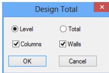
Press the command and in the dialog box choose the columns and/or the walls of the current level or the total building, to calculate the new [interaction diagrams M-N](#).
