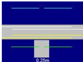
In the figure on the left, the positioned bars to the corresponding spans, pass through the spans on both sides, on the top and bottom of the beam.
