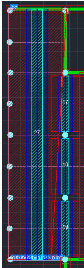
On the supported Line 27, the red right line has not formed correctly (it is the red inclined line). This happened because a support line was inserted which:
