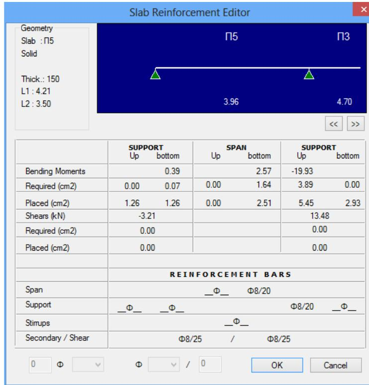
At the top left, you see the slab data such as name, size, etc. The dimensions are measured from axis to beam axis. Then the bending moments calculated for the supports and the corresponding span and the square centimeters of reinforcement calculated at the corresponding points are listed.
