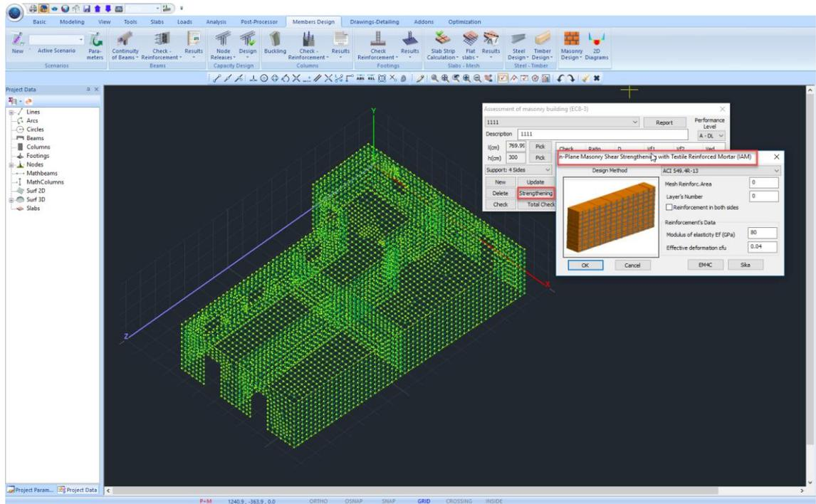
Use Textile Reinforced Mortar for shear reinforcement in the plane, defined by the corresponding window for the selected wall from the list.
