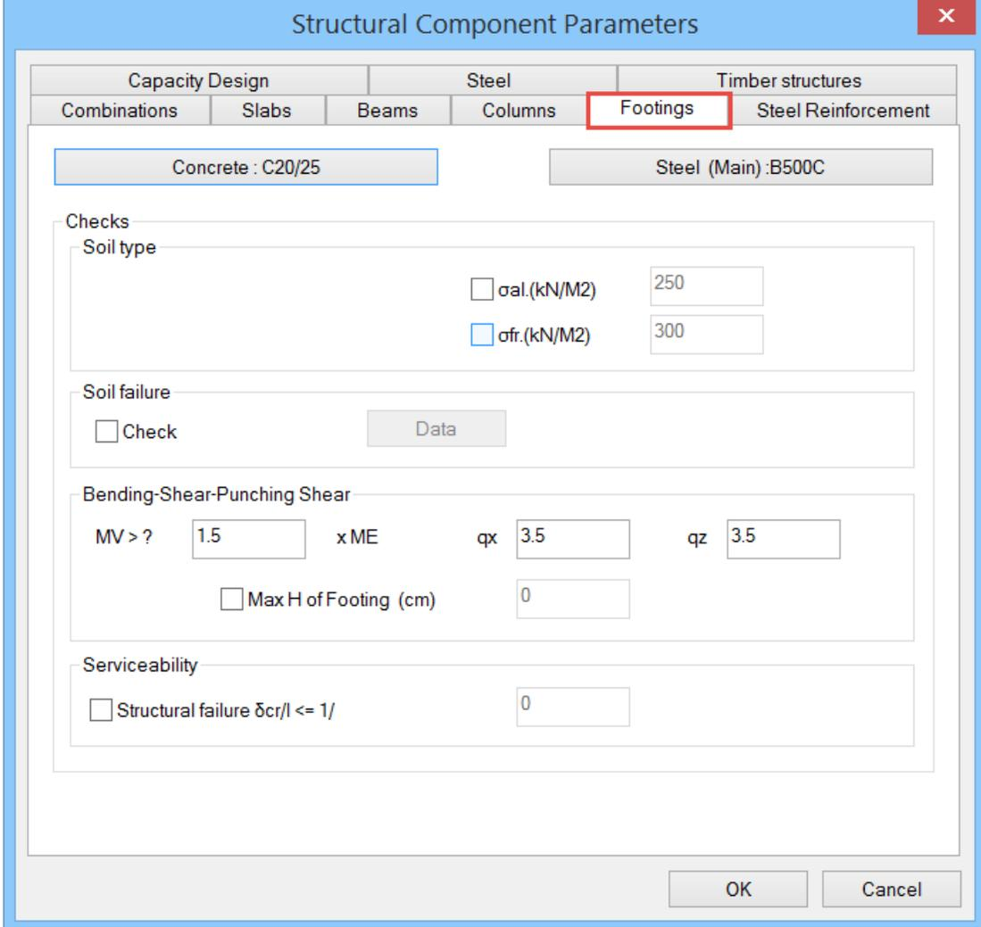
In the “Soil Type” field you can activate the checkbox  next to the relative stresses and type the value for the nominal stress  $\sigma_{al}$  (KN/m<sup>2</sup>) and stress fracture  $\sigma_{fr}$  (KN/m<sup>2</sup>).
