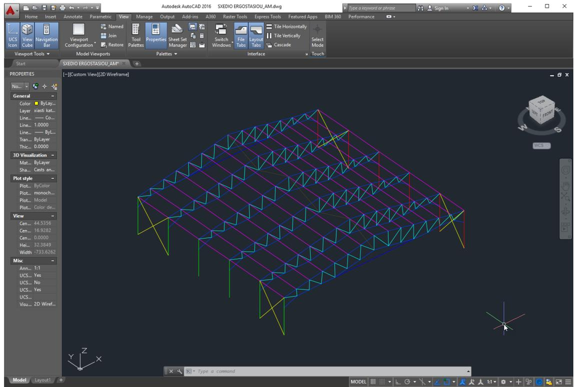
For this example, the design steel truss structure of the above image is used. It is a one opening frame structure with six trusses. In the 1st and 5th frame there are vertical wind bracings on both sides, and purlins on the roof.
