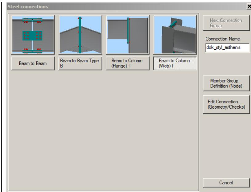
Left click to select the column member and then the beam member, and right click to open the library with the four possible types of connection. Select the last one “Beam to Column (Web)  $\Gamma$ ” along the main axis. Next set the name of the current connection.
