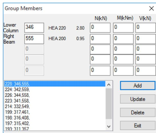
Use this dialog box for the design of steel connections with the same type and the same cross-sections in total.
