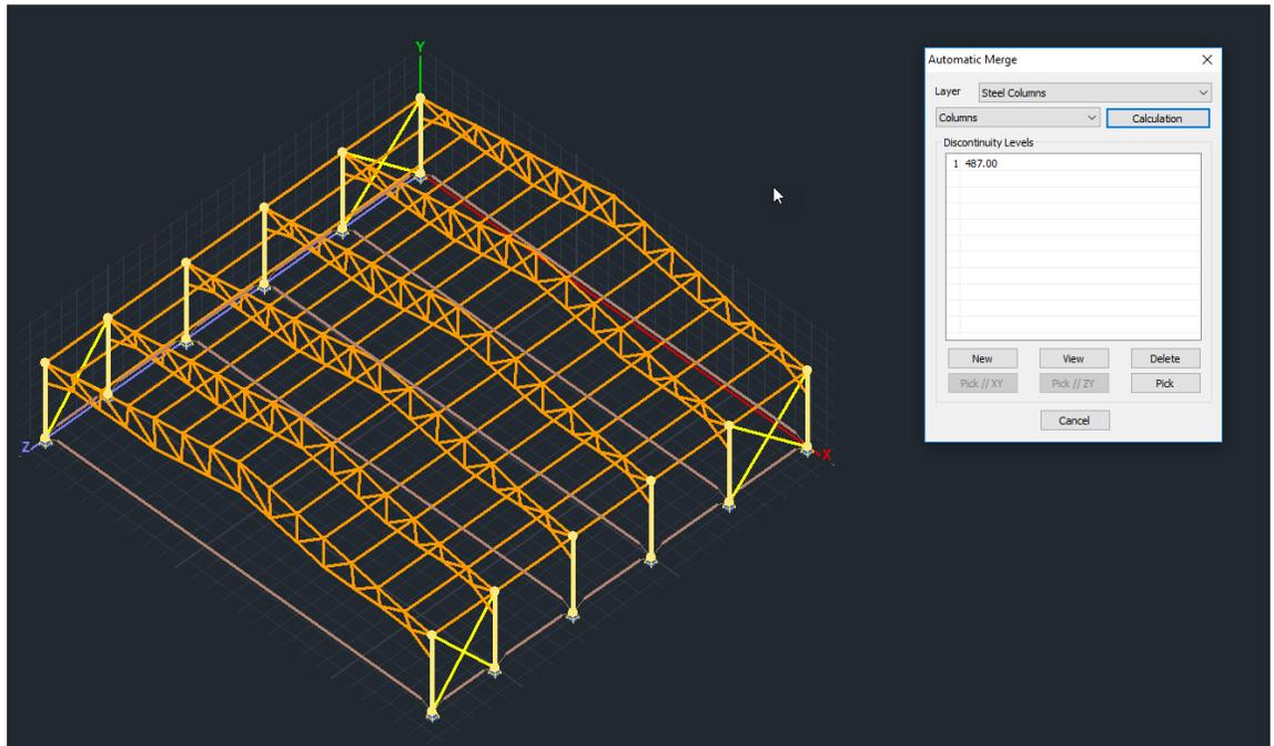
**Discontinuity levels** are levels that are boundaries of beams and columns, used to break merging in each direction.
