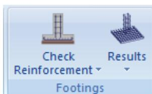
The “Footing” command group contains commands for footing design check, design calculation, editing and the respective results.
