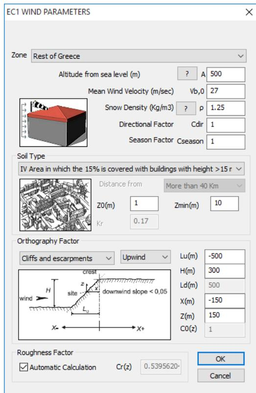
Select EC1 and define the Zone, the Soil Type, the Orthography and the necessary wind values. The Roughness factor is automatically calculated if the respective checkbox is activated, otherwise you can fill in a value manually.
