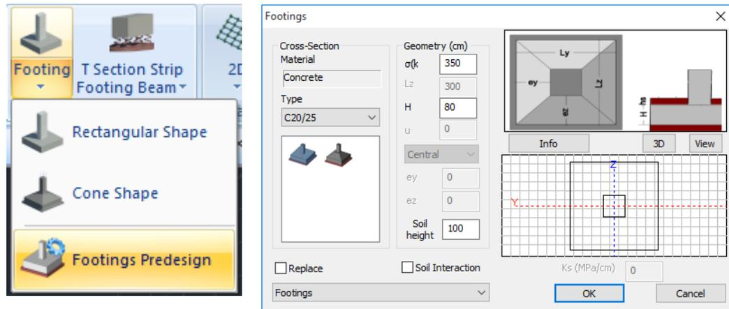
Which predesigns the footings and may change the dimensions of the footings by the soil interaction stress  $\sigma(\text{KN}/\text{m}^2)$ , the height of the footings  $H$  and the height of the supernatant earth  $h_s$ .
