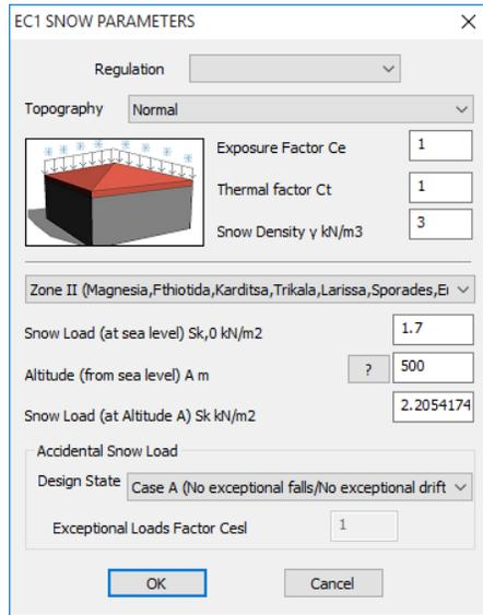
You set the topography which defines the values of the  $C_e$  and  $C_t$  coefficients, the Zone and the design state.
