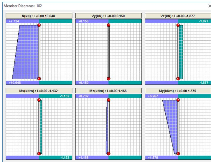
In this unit you can see over the members the diagrams of the stress on beam members and the stress/deformation/Reinforcement demand contours, for plate elements. For **Linear Members** you can see:
