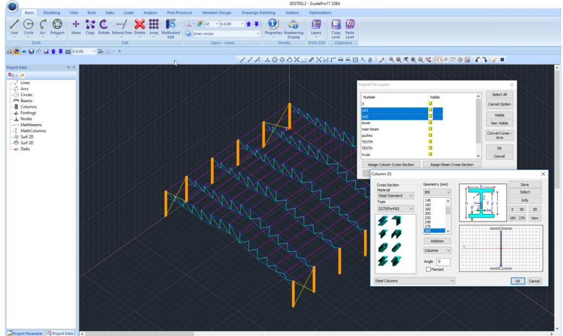
Repeat the same procedure for the Vertical Wind Bracings, selecting wind brac. and Assign Beams Cross-Section
