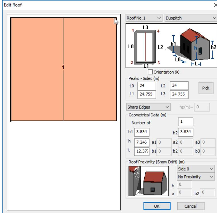
Define the type, the orientation and the dimensions  $L_0$ ,  $L_1$ ,  $L_2$ ,  $L_3$ , of the roof by clicking/button and showing with the mouse the four corners of the roof.
