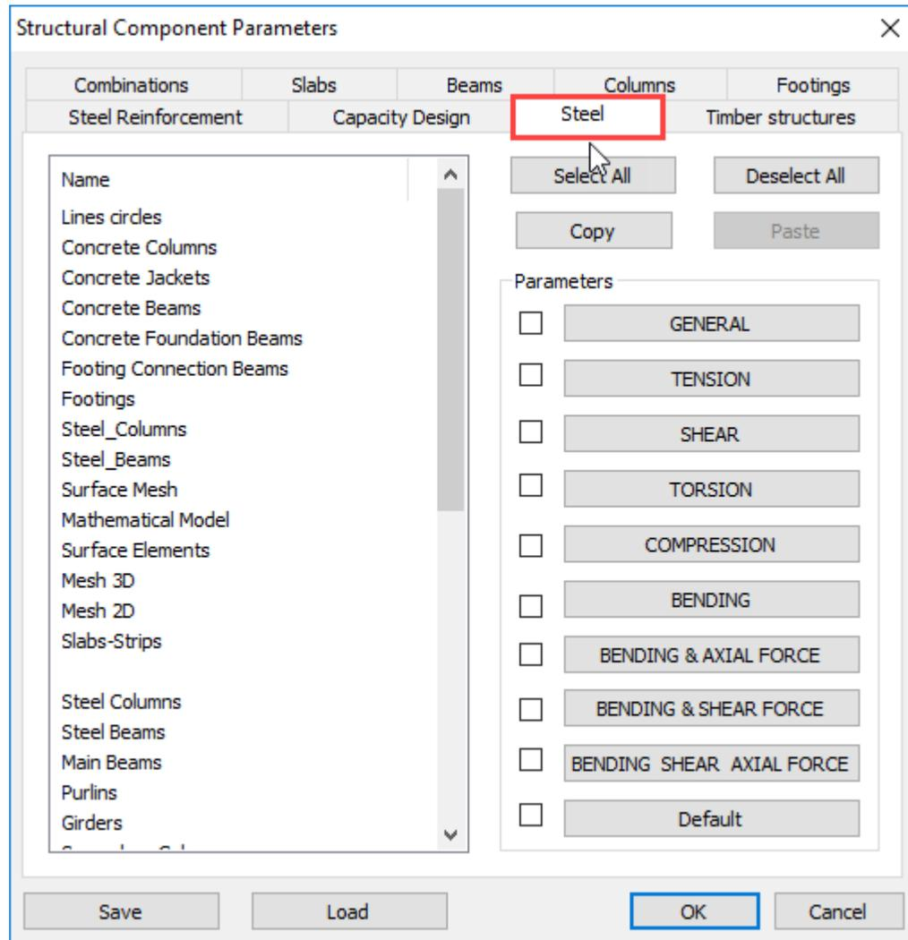
The definition of the design parameters for steel sections is performed per layer. First you select the layer of which the parameters are to be defined, (for example Steel Columns) and for each check category (General, Tension, Shear etc.), you set the respective parameters. As soon as you defined the parameters for one layer, the program gives you the ability to copy these parameters to another layer using the Copy - Paste commands.
