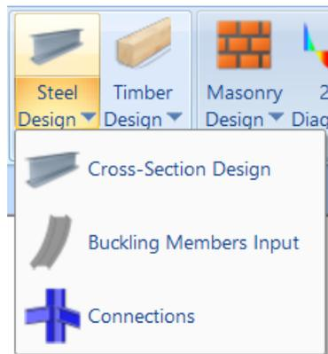
“Steel Design” command group contains commands for the cross-sections design, the buckling resistance and the steel connections design.
