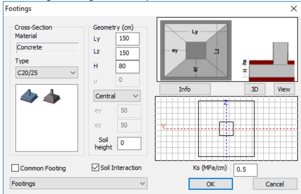
Use the 3D visualization to insert footings on the bottom of the columns elements.
