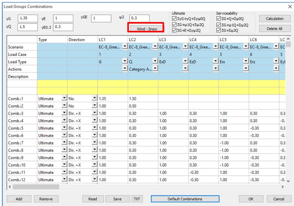
After running a scenario analysis, combinations are automatically generated by the program. "Combinations" opens the table with the combinations of the active scenarios.
