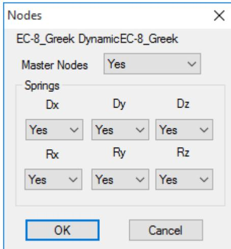
Here you can choose to perform the analysis without considering Rigid Link Constraint at any level even if master nodes exist and consider a fixed base for the whole model even if an elastic foundation is defined.
