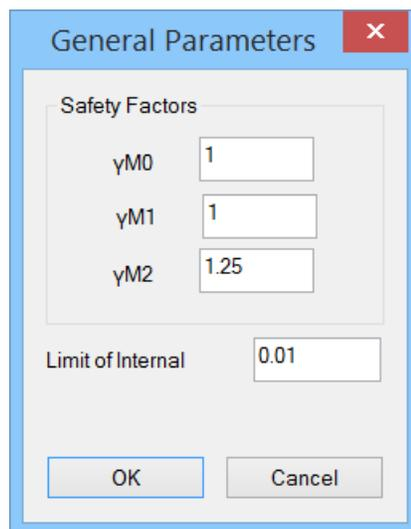
$\gamma_{M0}$ : partial factor for resistance of cross-sections whatever the class is
