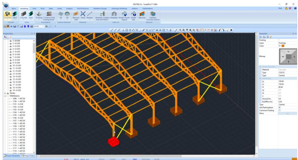
Correspondingly, for connecting beams, select the cross section and pass them from one node to the other, either in the Mathematical display or Physical. Automatically calculates the beams mathematical model:
