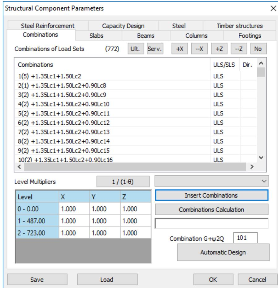
Prerequisite for the design is the calculation of the load combinations.
