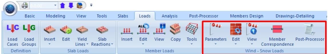
Through the “Loads” unit and the “Wind – Snow Loads” command group, the appropriate tools for the calculation and the distribution of the loads to the walls and the roofs, are located. The first step is to define the wind and snow parameters according to the location of the structure.
