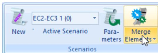
In the new version of the program, added a new command group, which concerns merging of steel (concrete and timber) members for the calculation and buckling and deformation checks display according EC3.
