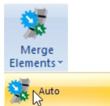
Merge elements means that, either automatically or manually, the individual parts of a single element, merge in each buckling direction.
