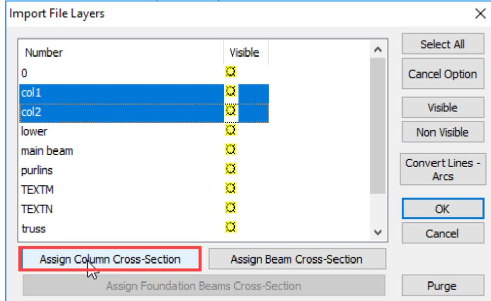
Set the section IPE300, angle 0, quality S275 and layer Steel Columns:
