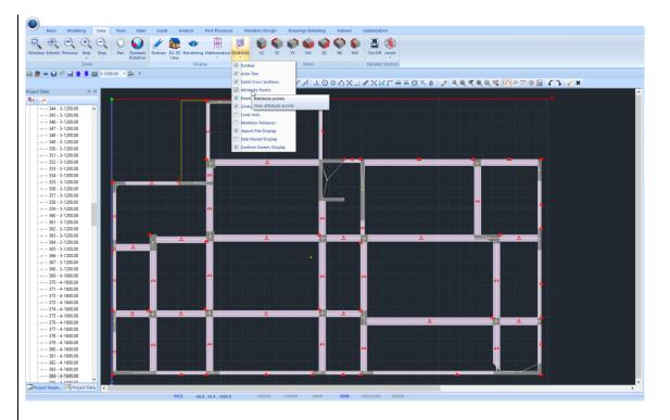
Using "Attribute Points" in "Tools" unit, you can modify the position of the Attribute Point in beams and columns.
