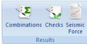
“Results” command group contains commands about the generation of the load combinations, the design checks, the analysis results and the seismic forces.
