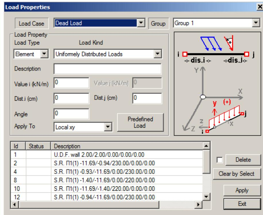
In the load list, you can see all the imported loads according to the selection. For example, select Dead Load/Group 1/Element/ Uniformly Distributed Loads. The list describes all the existing loads according to the selection. (U.D.F. Uniformly Distributed Force, S.R. Slab reactions)
