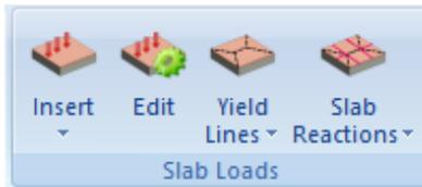
“**Slab Loads**” command group contains the commands for inserting, editing and assigning the slab loads on members and nodes.
