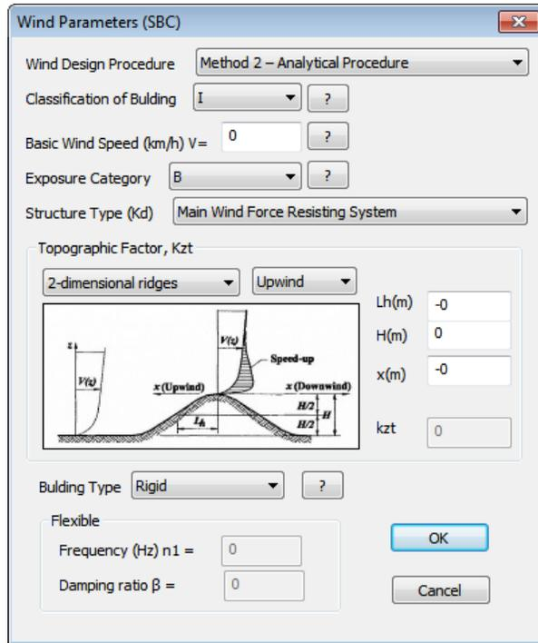
**SBC 301** provides three methods for calculating wind loads (par. 6.1.2)
