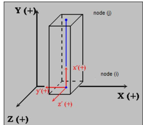
⚠ *Beams and columns local axes can also be defined using the rule of the right hand with your thumb along the positive axis xx, the index finger along the positive yy and the middle one along the positive zz.*
