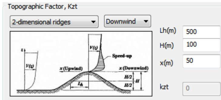
identifies the influence of the topographic configuration of the region where the structure is situated (FIGURE 6.4-2). According to these parameters, calculate the topography coefficient (Topographic Factor) Kzt.
