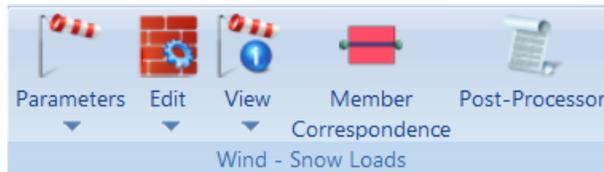
"Wind-Snow Loads" commands group contains tools for the automatic calculation of wind and snow loads and the distribution to members by Eurocode 1.
