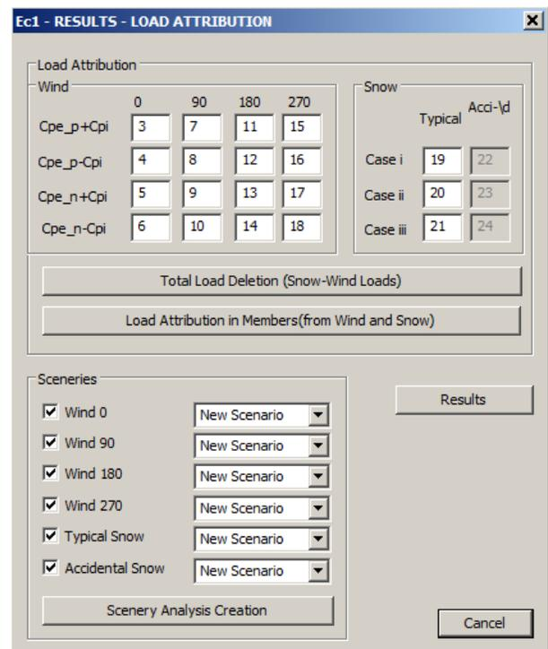
SCADA Pro not only calculates automatically the load distribution of wind and snow, but it also creates automatically all the analysis scenarios too, saving the user from hard work and much time.
