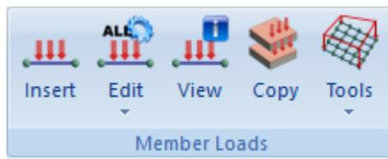
“Member Loads” commands’ group contains the commands for inserting, editing, viewing and copying loads of members, nodes and surfaces finite elements.
