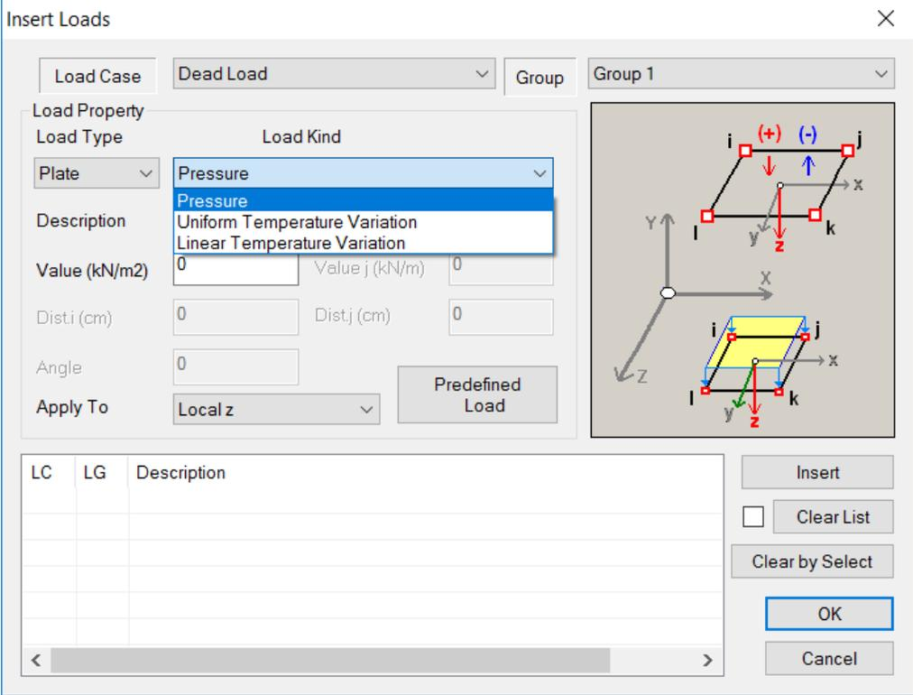
Allows you to define a **Pressure**, and also the possibility to enter **Temperature Variations** load for finite surface elements is added.
