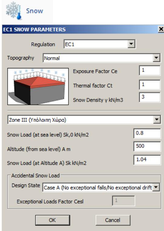
Select from the list the parameters: “Regulation”. “Topography” and “Zone” and the related fields are automatically updated. In the “Accidental Snow Load”: select a condition. Press “OK” to save the parameters.
