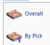
**Overall:** select the command (Load areas calculation for all current level slabs)
