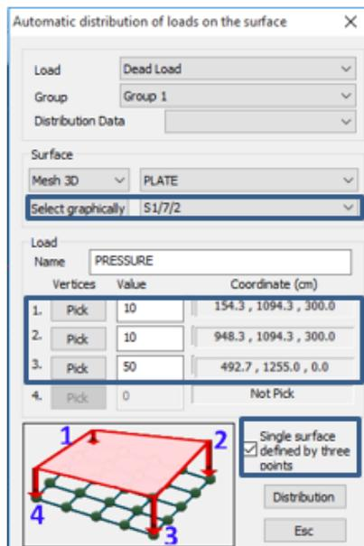
Check the option “Single surface defined by three points” and the 4<sup>th</sup> option is automatically disabled. Define the surface by pointing to the three points that define the surface using the **Pick** buttons. Fill in the pressure values (in kN/m<sup>2</sup>) and click **Distribution** and **Esc**.
