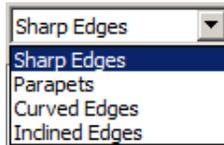
The user only needs to select **Inclined Edges**, and type in the height of the barrier in m and define the "Roof Proximity" as mentioned previously.
