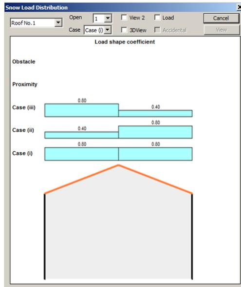
In the dialog box, select from the list the number of "roof" of the "opening" i.e. the number of the frame, (if there are more than one), and "Case"
