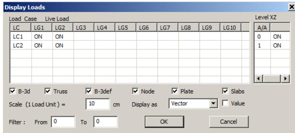
In the picture above there are two loads LC1 (Dead) and LC2 (Live). Each load contains a default group LG1 and a created group LG2, that are all “ON”, which means that all loads will be displayed.
