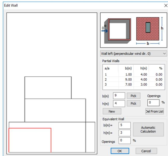
In above table fill in the geometrical characteristics of the "Sub-walls".
