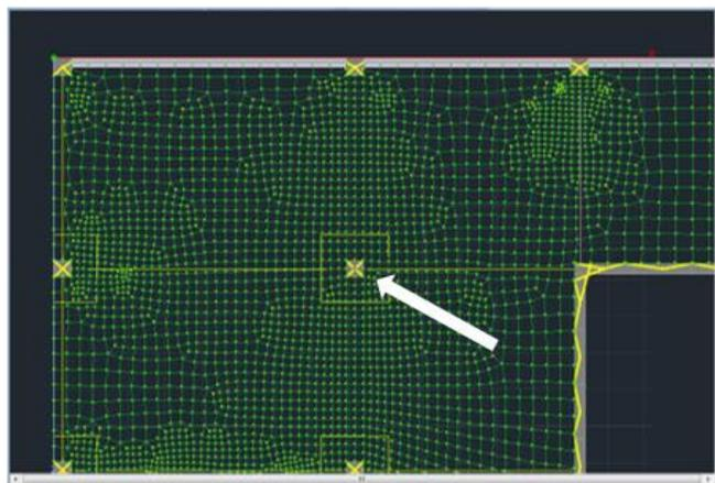
The punching shear check for this column gives a capacity ratio equal to  $0.291/0.356 = 0.81$ .
