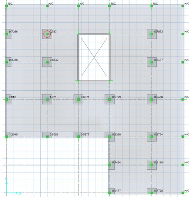
SCADA also computes a capacity ratio above 1.0 (equal to  $0.394/0.356 = 1.11$ ) meaning that punching shear reinforcement is needed. The results are presented below:
