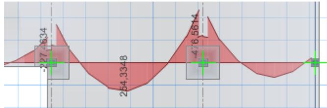
The corresponding value computed in SCADA Pro is equal to 245.990 kNm, that is a difference of about 3% in the values of the two software (the above value can be found in the folder scades\_FlatSlab of the project, file L\_14.txt).
