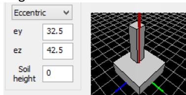
The button “**3D**”
