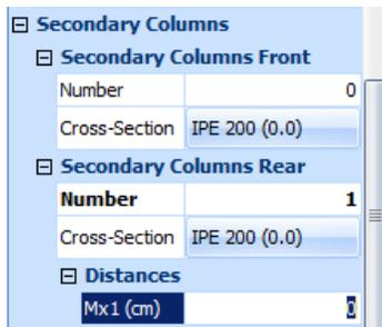
Type the number of the secondary columns (front and rear), define the cross section and type the relative distances. For a number different than 0, the "Distances" field opens in which you can set the distance in cm.
