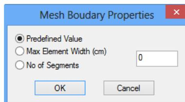
**“Predefined Value”:** This checkbox is used to define the number of the mesh elements. Type the number, click “OK” and then left click on the sides of the boundary. Right click to complete. Then select “3D” >> “Calculate” and the following dialog box appears:
