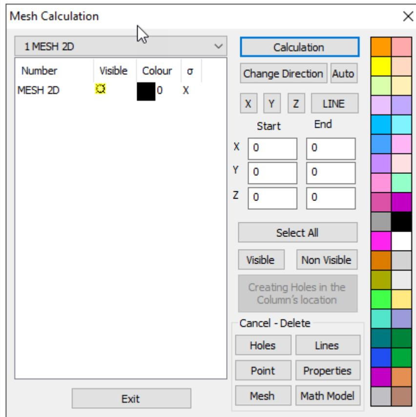
From the top list of the dialog box, choose the mesh group you want to generate. Note that each boundary must have its mesh group. This means that you cannot use "MESH 2D" in two different areas.
