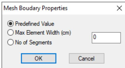
**“Predefined Value”**: This checkbox is activated to define the number of the elements for the total mesh. Type the number, click “OK” and left click on the sides of the boundaries. Right click to complete. Then select “2D” >> “Calculate” and the following dialog box opens:
