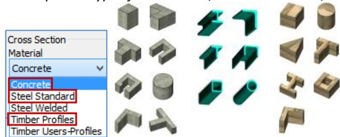
⚠ You can model Timber sections by following the same procedure, described for the concrete and steel sections.
