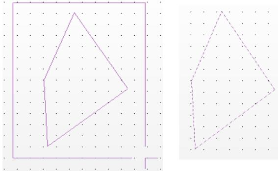
**⚠** Select again the command "Arbitrary Concrete Section" and in the dialog box, the cross section appears, with the input points and the local axes. To change the name, type the new one in the field and click "Rename".
