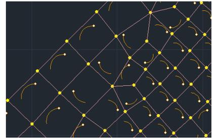
**⚠** Local axes, which are activated through the unit "View" >> "Switches" >> "Local Axes", are displayed on the elements after the creation of the mathematical model.
