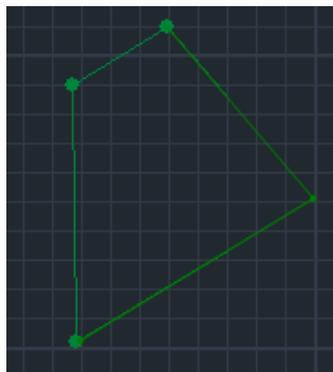
In the field **"Nodes"** you may type the number of the nodes of the single surface element, or type nothing and select the four nodes graphically, by left clicking. The element will be formed on the input interface.
