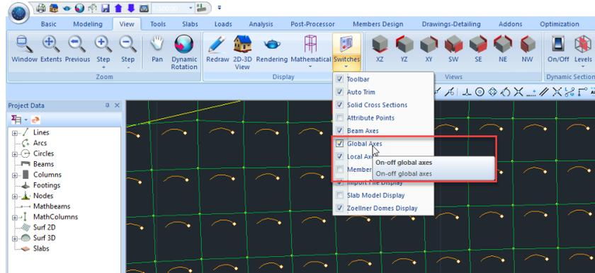
The arrows appearing defining local axes of the surface elements, according to the right hand rule. The direction of the arrow indicates the **x**-axis and the point on the edge indicates the orientation.
