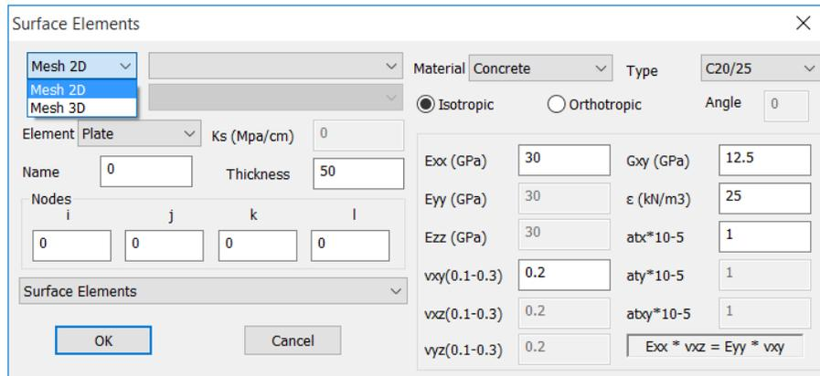
First, select the mesh type and the predefined surface. Parameters' fields are filled in automatically and can be modified manually.
