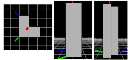
In the window below, you can see the formed section according to the geometry and the dimensions selected. You can also see the local axes yy and zz and you can change the insertion point (red point) by choosing a blue one.
