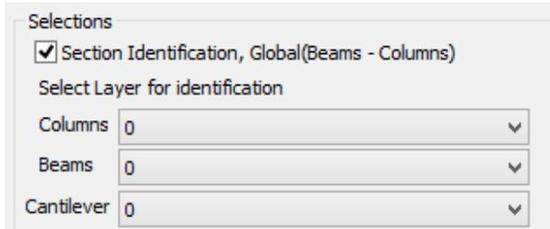
By activating the checkbox “**Section Identification, Global**”, all the elements (Columns, Beams, and Cantilevers) are activated for simultaneous identification.
