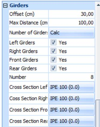
Calculate the number of girders as previously. Disable the direction without girders. You can choose different cross sections for the different girders' position.
