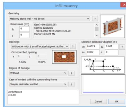
The data import process is identical to the one mentioned previously in the automatic process, except for the fact that you must enter by yourself the length  $l$  and the height  $h$  of the panel. Positioning the diagonal bars is a manual node to node process.
