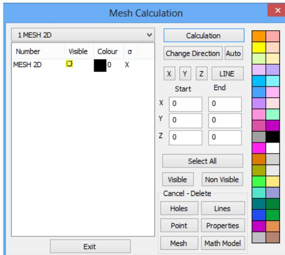
Select the Plate and then click the button “Calculation” for the mesh to be generated and to get the physical model of the surfaces.
