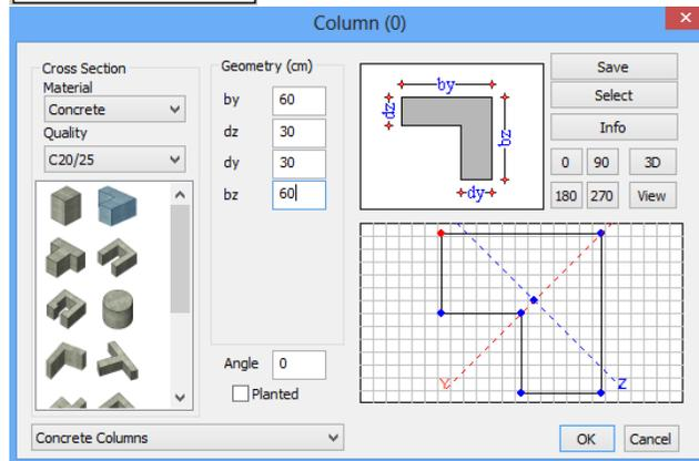
“**Cross Section**”: select the material (Concrete /Steel) and then the type. Choose a standard section from all the sections that appear, depending on the type of the material.
