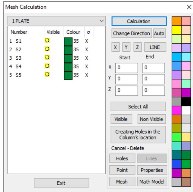
Select “Calculation” for the mesh generation and receive the following physical model of the surfaces.
