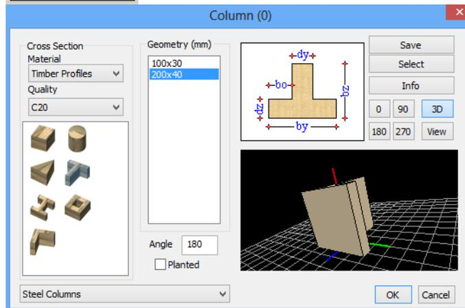
⚠ In the dialog box, all the sections are included. According to the selected material the respective type of the material, the cross-sections, and the geometry are displayed.
