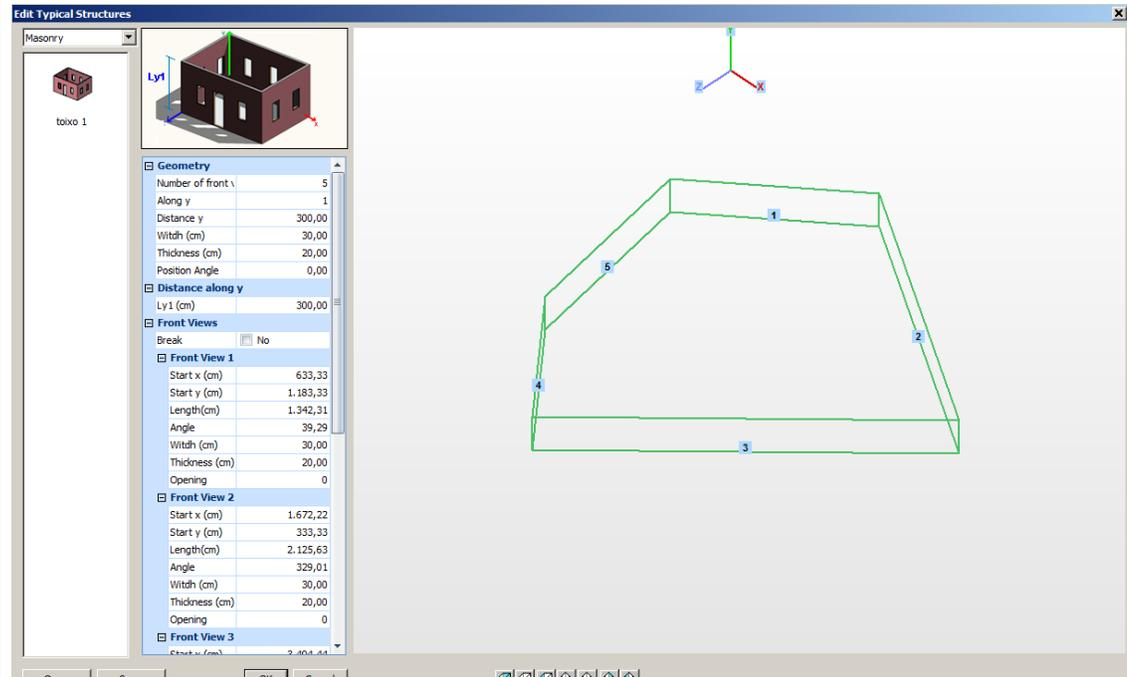
The program identifies automatically the geometry of the floor plan view. By default, the height is defined and the views are created according to the global axes.
