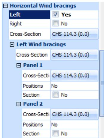
Activate the horizontal wind bracings of the left or/and the right side. The list expands further and for each panel, define the position and the intersection of the bracings. The same procedure is followed for vertical wind bracings.
