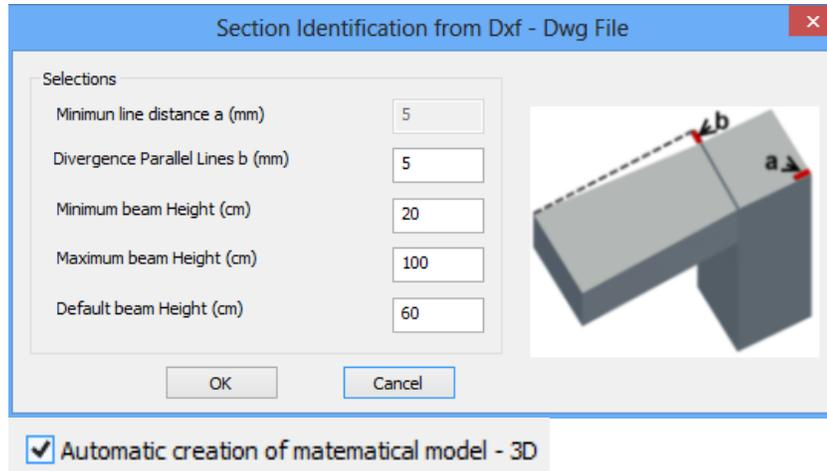
By activating the automatic creation of the mathematical model, the program not only identifies and imports the physical sections (physical model) but also calculates the inertial properties and creates directly the mathematical model too.
