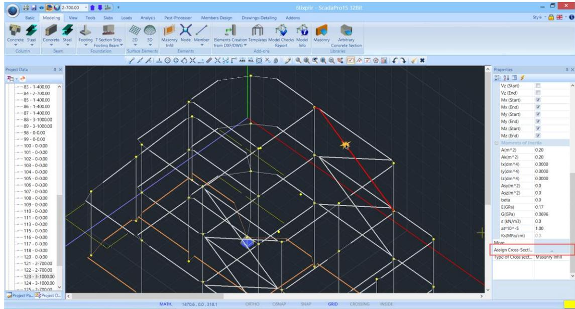
Left click on a diagonal member and in Properties select “Assign Cross-Section” to open the respective dialog box and make the changes.
