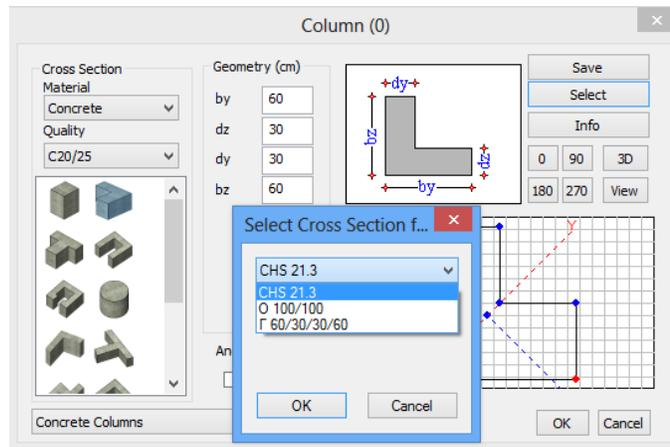
“**Info**”: This command is used to see the values of all geometric and inertial data of this section.
