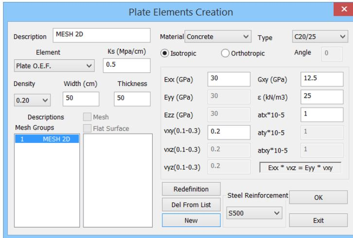
If you don't need to make any change, go directly to “Modeling” >> “Mesh 2D”>>“Calculate”, and the following dialog box is displayed:
