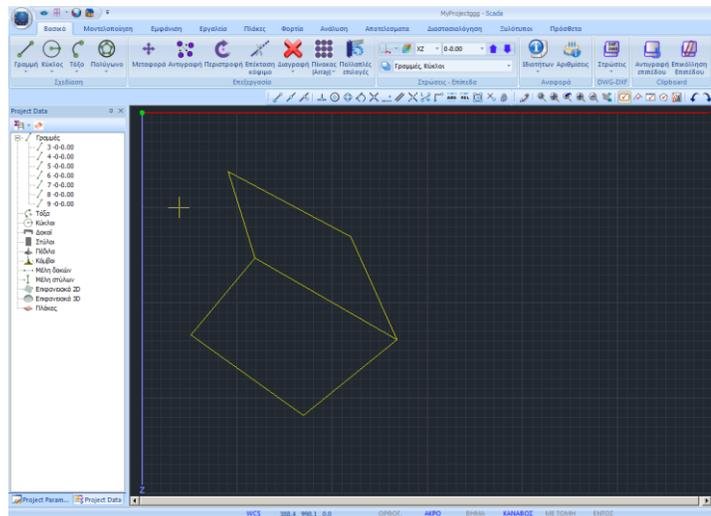
Use “Modeling” >> “Surface elements”>>”3D” >> “Mesh”, to define the mesh:
