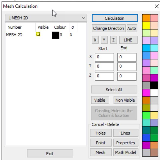
Select a mesh and click “Calculation”. The number of the elements of the mesh will change and the mesh will be updated based on the predefined value.
