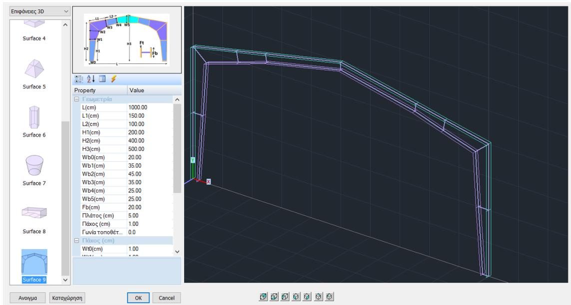
SCADA Pro provides multiple possibilities for using 3D surface elements, through "Templates" and the command "Front view identification", which is explained in detail later in this chapter.
