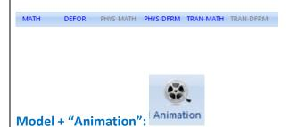
"Animation" command is a button that activates and deactivate the deformed structure of animation, according to the selections made in "Deformed Model" dialog box.
