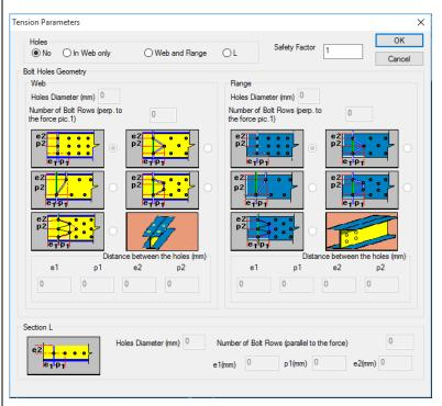
Specify the spacing of the centers of two consecutive holes, the diameter of the hole and the number of rows of bolt holes.
