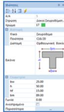
The list of Properties that appears on the right is automatically filled when an existing element is selected. It contains information about the properties of the structural element and allows the user to modify easy and quickly those properties.
