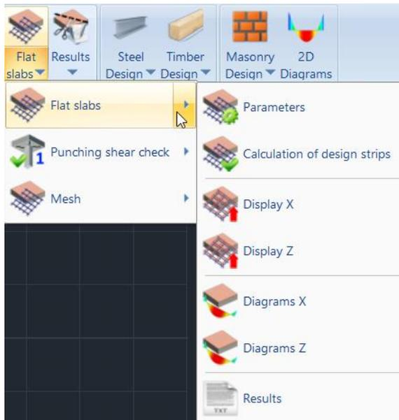
The new version of SCADA Pro offers the possibility of creating flat slabs (slabs without the presence of beams) with the finite element method.
