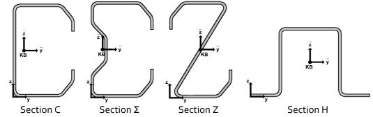
The cross sections may be either not reinforced or have single or double end reinforcements (see figure below). The bending angle of the reinforcements and the trunk of the Z sections are also parametrically defined.
