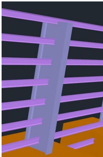
The local axes direction of the column and the girders are as shown in the figure below:
