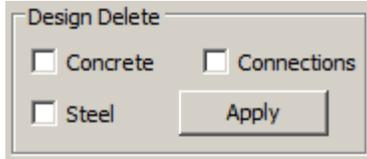
In the field “Design Delete” activate the corresponding checkbox and then press “Apply”, to delete the results of the previous design checks. Repeat this procedure using other combinations or parameters or scenarios, etc.
