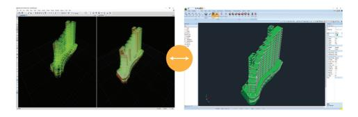
The new bi-directional communication of SAP2000 and ETABS with SCADA Pro, allows export and import of any project in SCADA Pro and SAP2000/ETABS, respectively.
