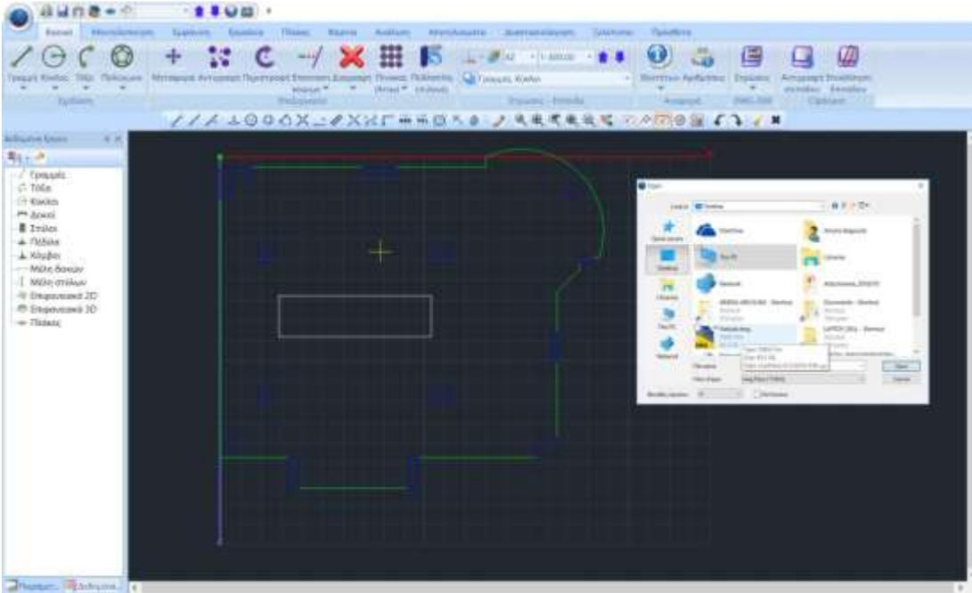
4. With the Layers command we convert the lines of the pillars and the outer contour of the auxiliary to Scada lines.
