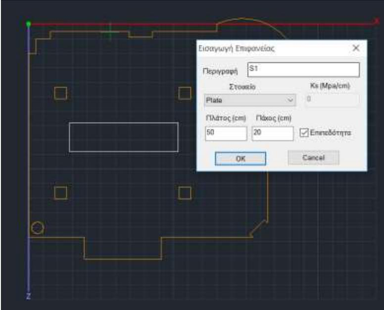
In case the perimeter at any point is not closed, an **X** will appear on the screen at that point.
