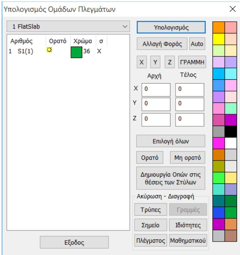
However, in addition to the central hole, there should also be holes in the position of the inner posts. These holes are automatically created by selecting the command
