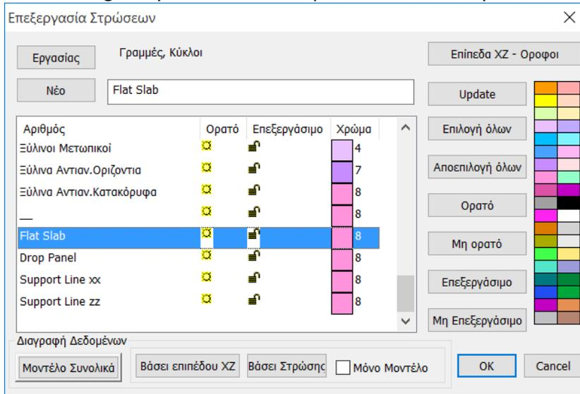
Scada's default list of Layers includes the layers related to the Flat Plates.
