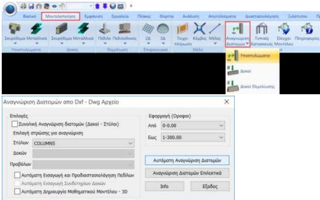
The cross-sections of the poles belonging to the corresponding Layer are automatically identified.
