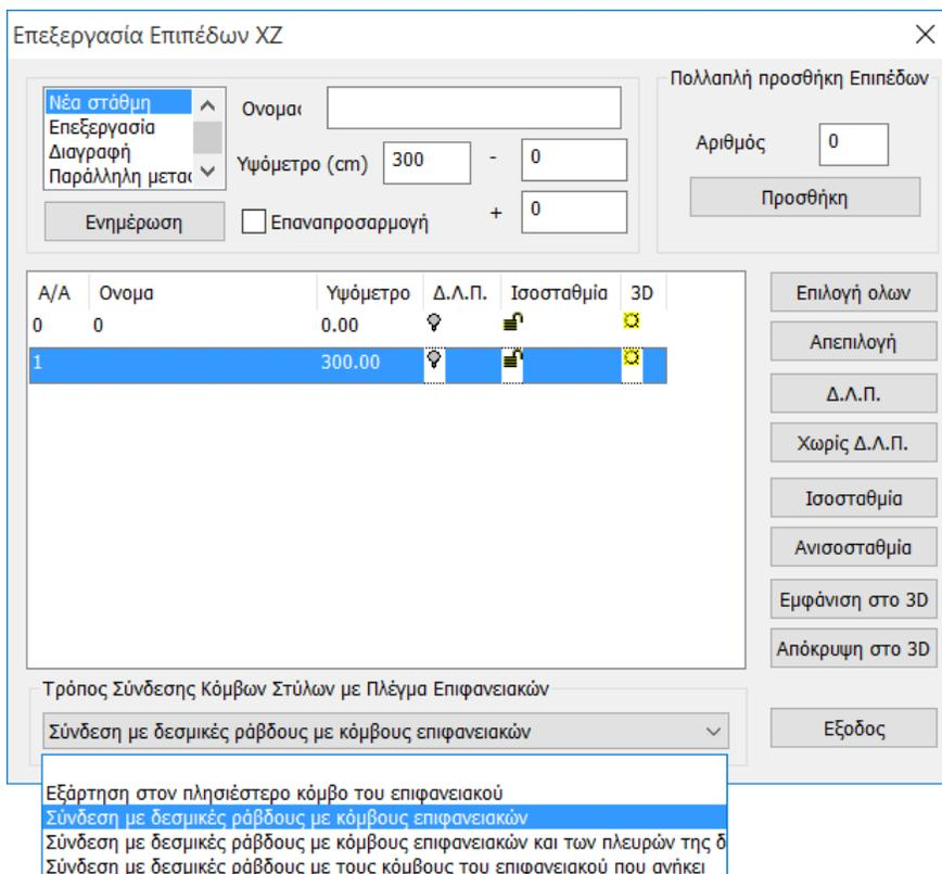
At the bottom of the window there is a choice of the way of connecting the nodes of the columns with the surface grid, for the selected level, we choose the connection with tie rods and with the nodes of the surface grid. At the end we press Update.
