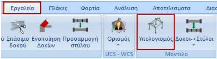
To create the mathematical model of the vector, from the "Tools" section select the command "Calculate" and press the OK button in the dialog box that opens:
