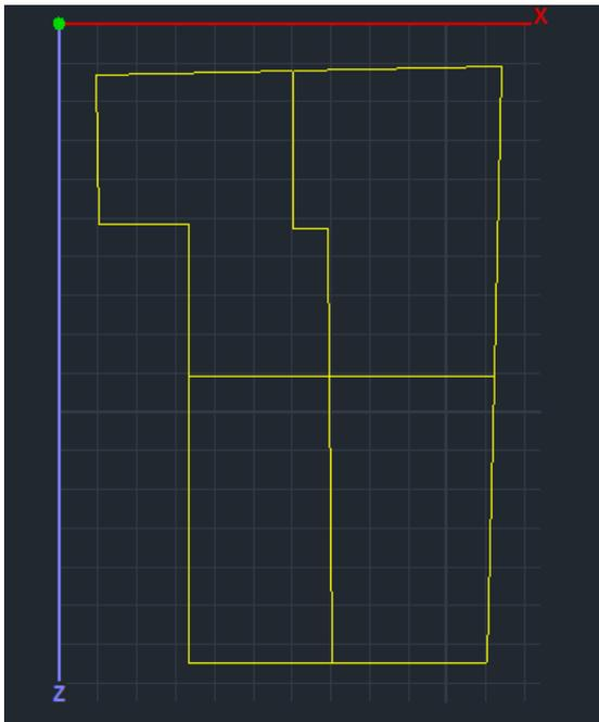
In the Modeling section, select the command "3D External Boundary, with the left mouse button point successively to all the contour lines of each plate and finish with a right click.
