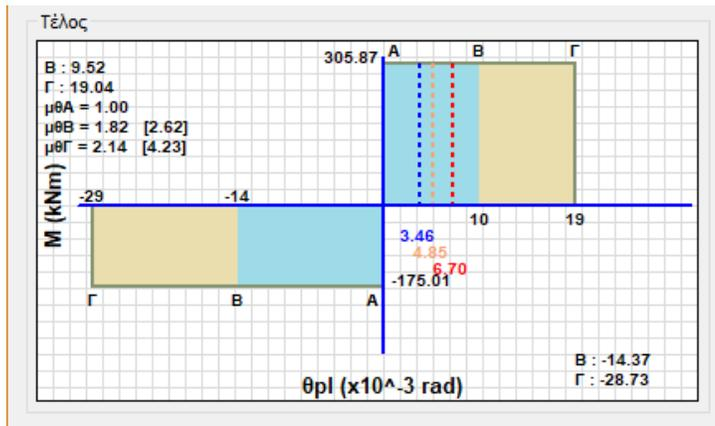
The yellow colour means that the corresponding value (orange line) has entered the brown area and the corresponding red one has not left the brown area.
