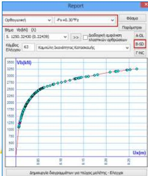
You select the type of distribution with which the control and sizing of the reinforcements and the level of performance will be carried out and by referring to the "Steps", you locate the post where the first plastic joint will be carried out.
