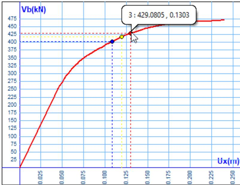
Moving the mouse to the points Displays the values for the three targeted movements, one for each performance level and the corresponding intersections at the Control Node.
