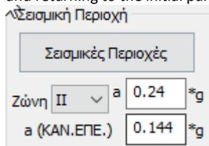
we see the value of the ground acceleration as it was calculated previously and as it will be used in the execution of the scenario for the calculation of the seismic action.
