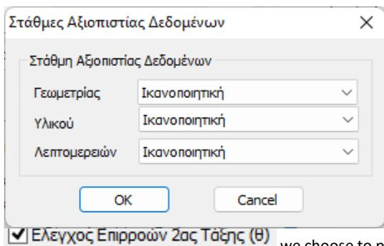
for the existing building according to the provisions of the CEE. This choice affects the coefficient of permanent loads  $\gamma_g$  on the basis of which the building will be solved.
