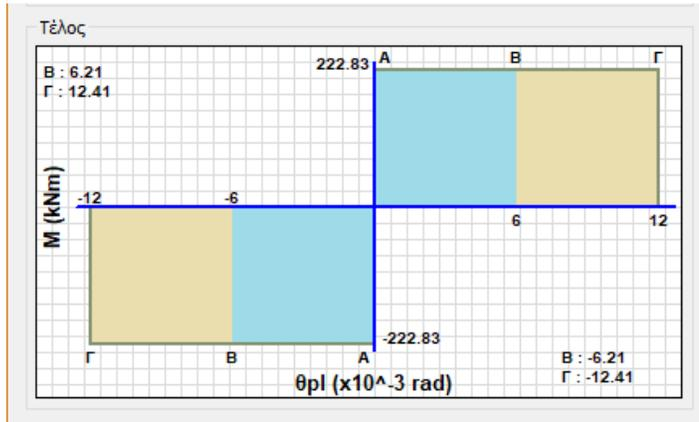
The blue colour means that: the corresponding blue line is within the blue area, i.e. the limit of A (which is 0) has been exceeded, but both it and the other two values have not exceeded the limit of B (blue area).
