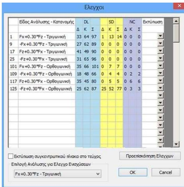
This table gives you, each inelastic analysis performed, the total number of insufficient beams and columns for each performance level.
