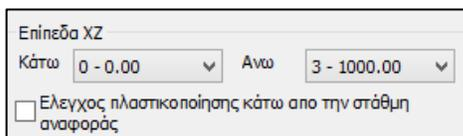
You define from which level to which level the horizontal seismic load will be applied. It is suggested that the upper level be defined as the last full level (not staircase ends). This level will include the control node, which will be either the bulkhead node or another node on the outer perimeter of the building.
