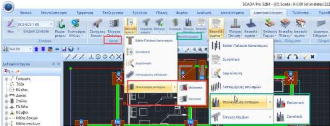
It involves the calculation and display of the moment-axial interaction diagrams, based on the geometry of the cross-section, the quality of the materials and the reinforcement. The three-dimensional diagram of the strength envelope ( $M_y$ ,  $M_z$ ,  $N$ ) is produced. In addition, the Tension-Deformation diagrams for steel and concrete are displayed schematically, and the Stress-Curvature diagram is shown in detail.
