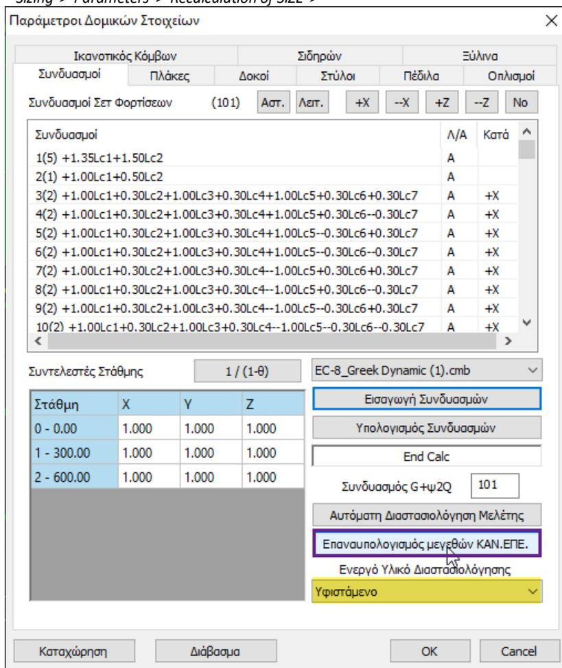
Through this command, the program calculates the M-N interaction diagrams for all structural elements of the beam
