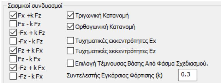
We define the combinations for which inelastic analyses will be performed. Each combination means that a seismic force will be applied in the specific direction (x or z) with a factor of 1 and a seismic force in the transverse direction with a factor that you specify in the "*Transverse load factor*" field.
