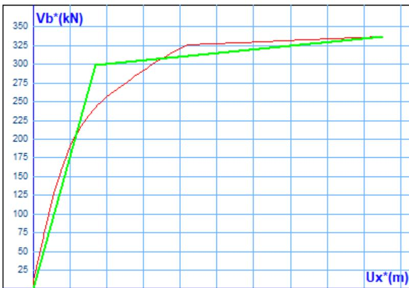
The key  button to define the parameters for the bilinearization of the construction capacity curve. This bilinear curve is necessary so that the slopes of its two branches can be used to calculate the eigenperiod and the corresponding spectral acceleration.
