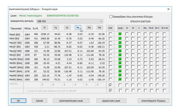
In this example, the adequacy ratios are much smaller than unity. This means that we could use smaller cross-sections.
