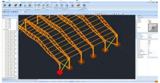
Similarly, for the connecting beams, you select the cross-section and pass them from node to node in either Mathematical Illustration or Physics. Automatically you also calculate the Mathematical Model of the beam:
