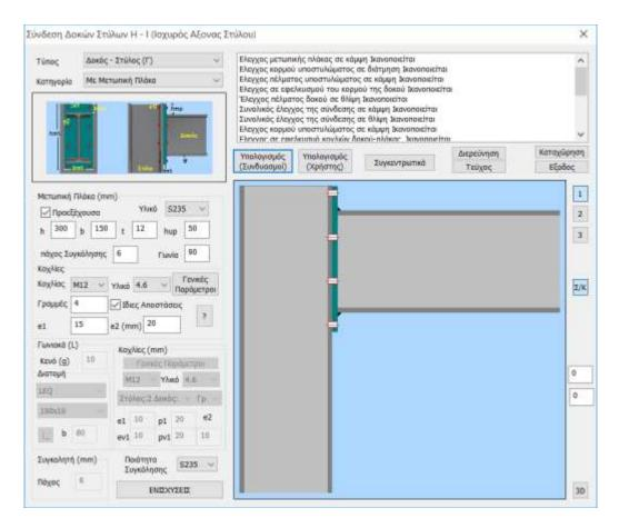
If you click on the 3D command (bottom right) you will see a three-dimensional representation of the connection which is dynamically updated as you make changes to the parameters. Buttons 1, 2, 3 correspond to side view -1, side view -2 and plan view -3 and via the S/C command you can display in the 3D view the welds and bolts.
