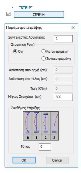
Here you specify whether the members of the layer are loaded by torsional moment (distributed or concentrated). If they are loaded, you define the elements of the loading. You also specify the support conditions of the members based on the support type shown in the graph.
