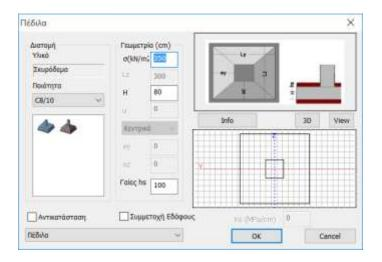
which, according to the soil tension  $\sigma(KN/m2)$ , the height of the footings H and the overlying soil hs, pre-standardizes the existing footings, possibly modifying their dimensions.
