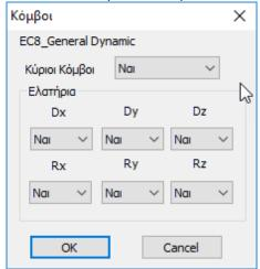
Here you can specify to resolve your girder without diaphragm mode altogether, even if there are diaphragm nodes, as well as to resolve it pressed (Spring No) even if elastic foundation is set.
