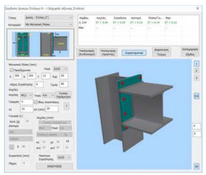
When the checks of the geometry and topology of the connection are satisfied, the program will make all the required calculations and display all the checks performed according to Eurocode 3 for the specific connection.
