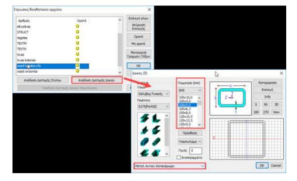
Set SHS100X5 and assign it to the layer Metal.Vertical. Ok, and the cross-sections of the abutments are automatically imported.
