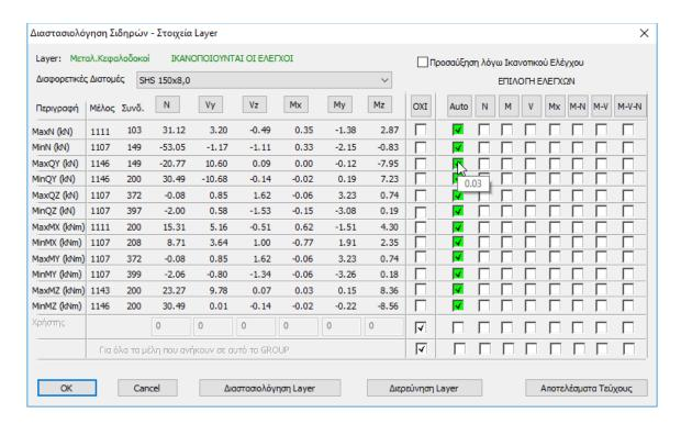
Moving the mouse to the green indicator, we see that the adequacy ratios are very small and that there is room for reducing the cross-section.
