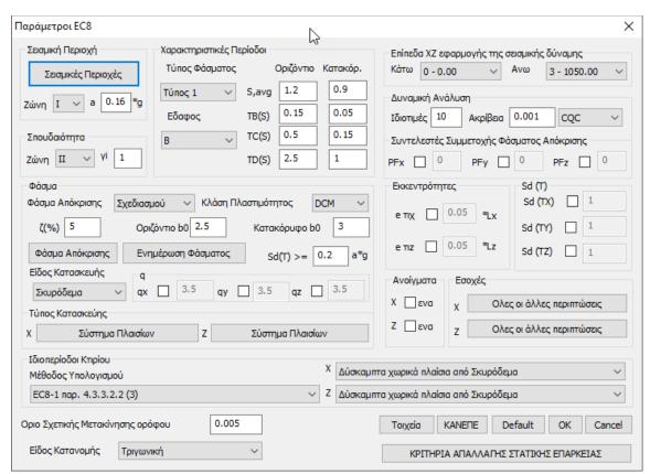
In this dialog box, enter the necessary information about the seismic area, the terrain and the importance of the building, as well as the earthquake application factors and levels.
