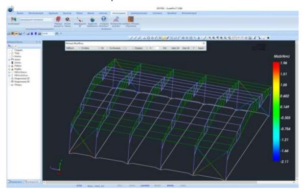
In this section you can see on the members the diagrams of the stresses for the linear members, and the isometric curves of stresses, strains and reinforcements for the finite surface elements. In particular, to see for the Ribbon elements
