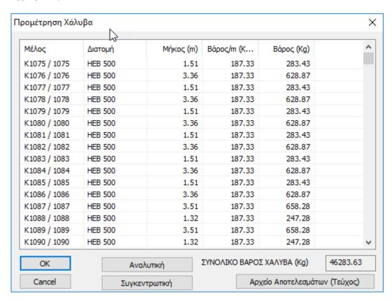
SCADA Pro enables you to have a detailed premeasurement of each steel section by member or an aggregated premeasurement by section category.
