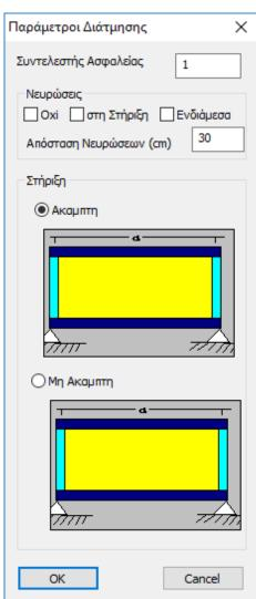
Here you define whether the elements of this Layer have ribs or not and if they do, where they are present (on the support and/or the trunk). You also define the spacing of the ribs as well as whether the support of an element is rigid or not.
