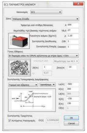
You select EC1 and indicate the Zone, Land Type, Topographic Configuration, and the necessary wind values.
