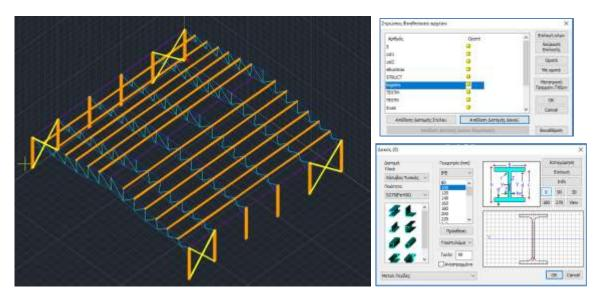
For the mesh elements, define three New Layers within the "Edit Layers" window:
