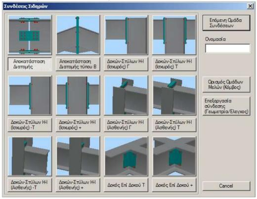
B) Alternatively, you can click on the "Links" command and then left-click on the members you wish to link. Right-clicking then displays a window in which only possible connections consisting of only two members included
