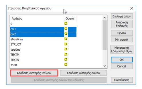
Set cross-section HEB500 with angle 0 quality S275 quality and layer Metal. Support columns.
