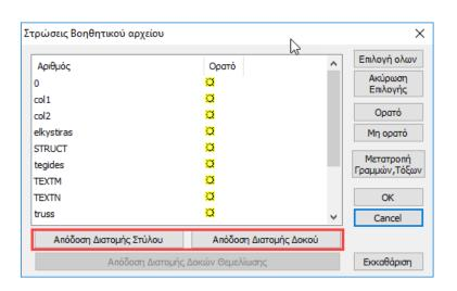
Select the Layers col1 and col2 and press the Column Cross-section Performance button
