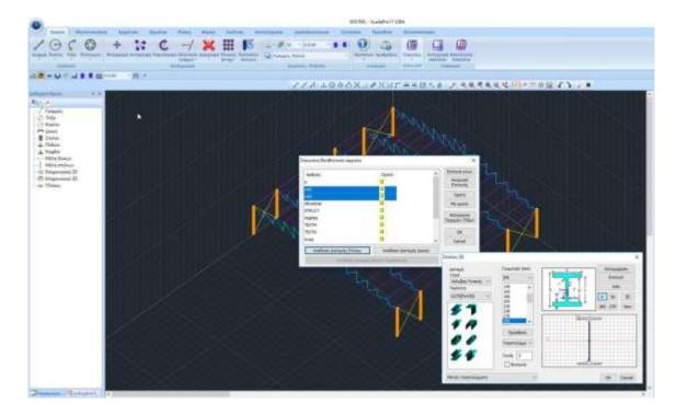
The cross-sections of the columns are automatically inserted in the position defined by the lines of col1 and col2 layers of the auxiliary file.
