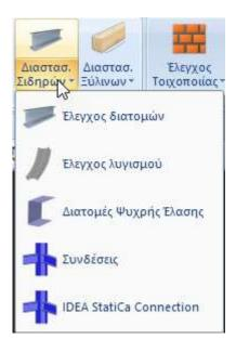
In the "Dimensioning" module, "Iron" field includes the commands related to the solution of the metallic sections with the adequacy check, the buckling check and the check of the connections.
