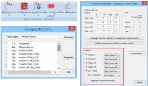
Subject to the above conditions, it is possible to create the wind and snow combinations automatically using the Aνεμος - Χιονι command.
