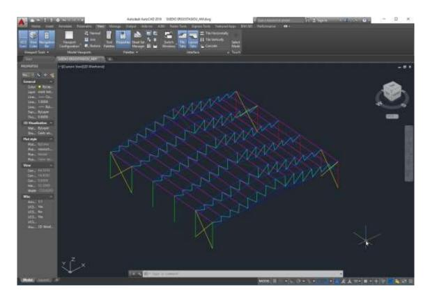
For this example, the design of the network in the above picture is used. This is a single opening grid with 6 meshes. In the 1st and 5th frames there are chiasm windbraces on both sides, and purlins on the roof.
