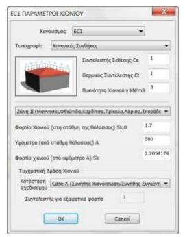
Specify the Topography that determines the values of the coefficients Ce and Ct, the Zone and select for Greece Planning Condition A.
