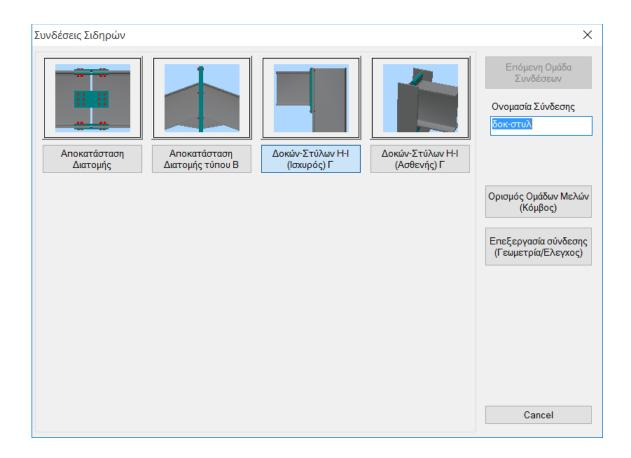
For example, select member 30 (column) and member 154 (beam) in sequence. Right-click to display the window with the 4 possible connection types. Select the last (to the right) connection which corresponds to a Beam - Column connection of cross-section type H or I on the strong axis. You will then enter a name for this connection.
