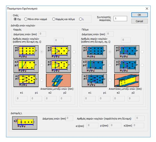
For the holes define the distances from the ends, the diameter and the number of rows on the torso and tread.
