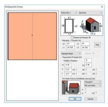
define the type of roof, its orientation and the dimensions Lo,L1,L2,L3, by pressing Pick and selecting each time with the mouse the 4 edges of the roof, as well as the Geometric Elements.
