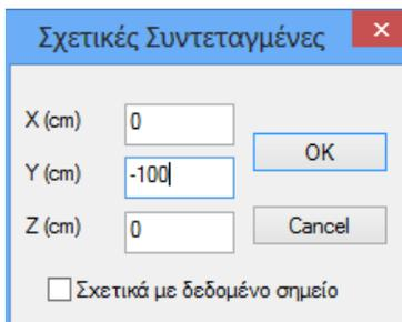
In the "**Relative Coordinates**" window, write in cm the relative offset and click "**OK**". Automatically the nodes are lowered and the slope is created.
