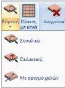
With the command "**Find**">"**Total**" the program automatically detects all closed contours present on the level and automatically enters all the slabs of the floor.
