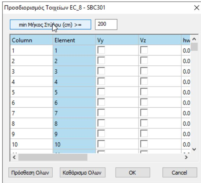
Enter the min Length (cm) and press the command "min Column Length" to automatically determine the walls per direction, so that the calculation of T1 is done according to par.4.3.3.2.2.
