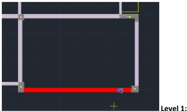
You can repeat the same procedure on the foundation level or copy these new columns of level 1<sup>th</sup> to level 0 using "Copy" command.
