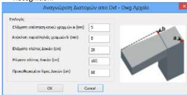
For the identification of the beams, the limiting distances of two lines in the layer of the beams are defined, as well as the predefined height, i.e. the hanging of the beams that the program recognizes from the floor plan and always enters with a rectangular cross-section.
