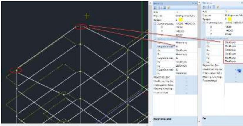
In addition, to simulate a sloping slab or roof slab diaphragm mode , you can multiply the  $I_y$  of its perimeter beams by a factor (50 to 100).
