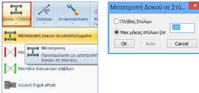
First you draw the mathematical model of the beams that will be converted into basement walls. Then you select the command and left click on the level 1 beams to be modified and automatically the program converts them into successive columns.
