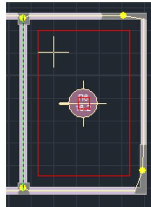
Two parallelograms are automatically formed, a smaller one, which is the gap with the dimensions you specified, and a larger one, which is the inner boundaries of the solid zones. Select one vertex of the gap (small par/me) and then one vertex of the large one, from which to start placing the gaps.
