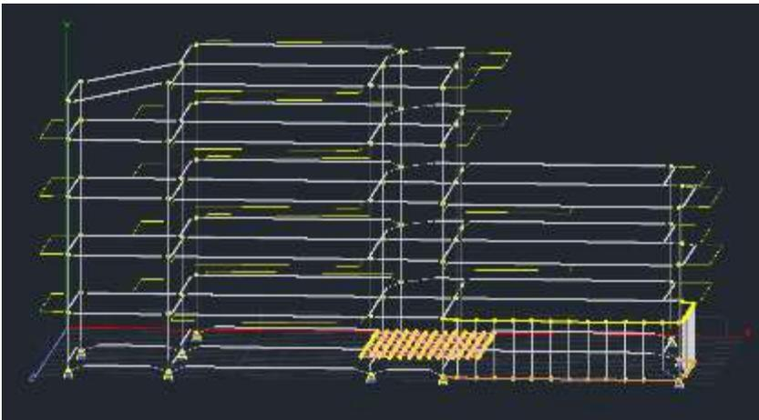
In order to be able to enter the sections of a slab, it is necessary that its static elements (beams-pillars) belong to the same level. So in the case of a sloping slab you must define the unbalance of the floor to which it belongs:
