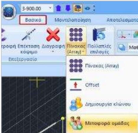
From the "Basic" section select the "Group Transfer" command, activate the "With window" option and enclose the node and right click.
