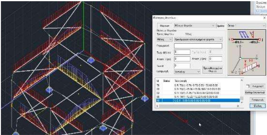
In this way, you can better control the loads that have been applied to the elements of the structure and that will be affected by a possible overall modification.
