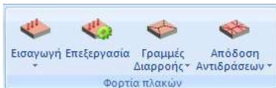
From the "**Plate loads**" field, select "**Insert**". You have the option of entering loads, either in total for all slabs of the active floor, or selectively for one slab at a time.
