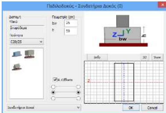
In the dialog box set the characteristics of the material and geometry of the beam and the insertion tolerance<sup>(\*)</sup>.
