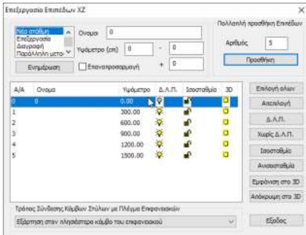
At the bottom of the window there is the choice of the way of connecting the nodes of the columns to the surface grid, for the selected level, by selecting one of the three ways, connecting the nodes either by simple dependency or by connecting through tie rods.
