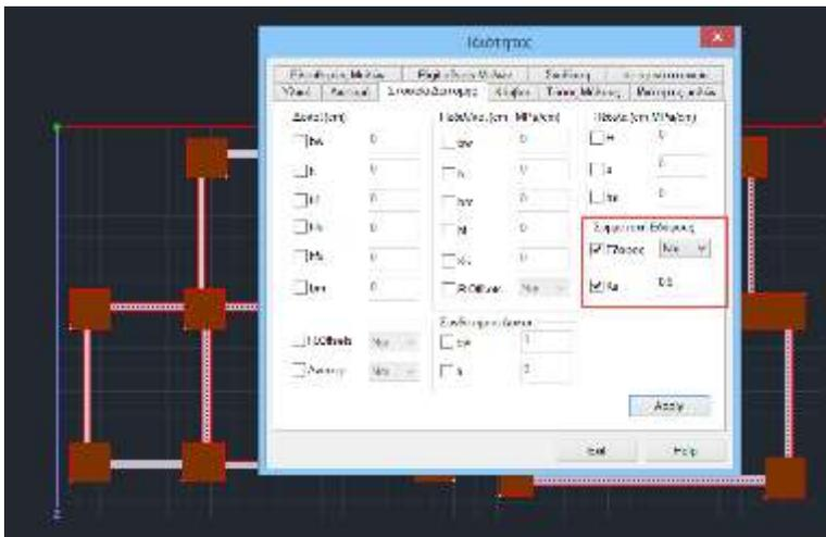
Left-click to select a node of a pedestal and check in the properties that the change has been made.
