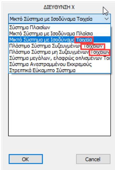
then to calculate the coefficient  $\alpha_0$  and ultimately  $q$  you should select the "Tunnelscommand **Τοιχεία** to define, based on a minimum length, which of the vertical elements are defined as "Tunnels".
