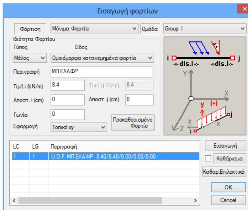
By selecting the "*Insert*" button, the defined load is displayed in the table with all its elements and with OK it is applied to the selected members.
