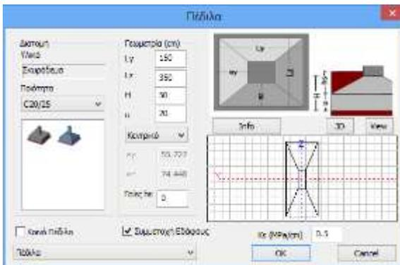
In the dialog box set the characteristics of the material and the geometry of the pedestal. Click on "OK" and place the skirt on the desktop by left clicking on one of the sides of the superstructure column at level 0. Repeat the process to insert the remaining sandals.
