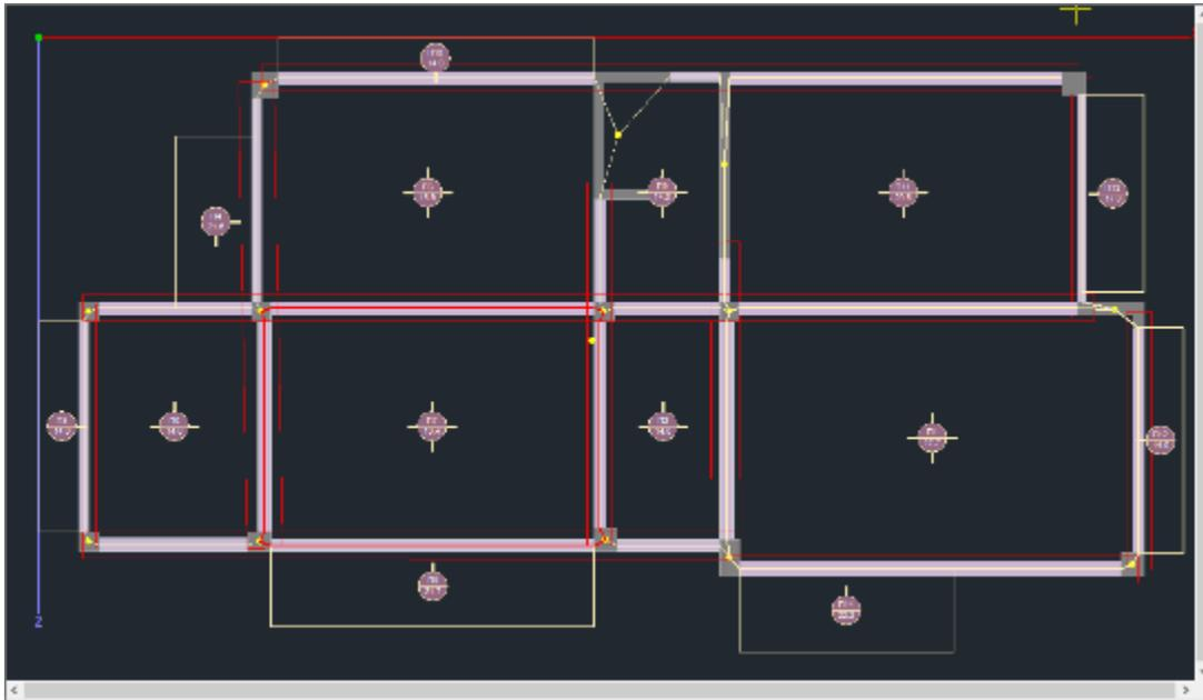
In "Arming Preferences" you specify whether one or two reinforcement bars will be placed as common support reinforcement in the beams, whether you wish to take into account the bars of both openings in the support reinforcement, as well as the anchorage length by varying, if you wish, the support width of the beam.
