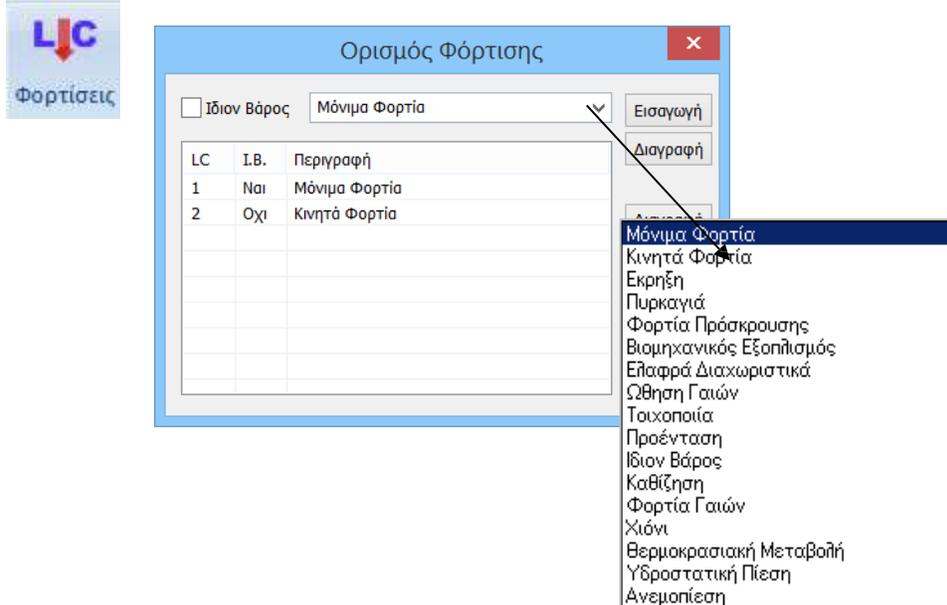
The dialog box includes by default the two main loadings, Permanent and Mobile. The user has the option to delete ("*Delete*") or insert other loadings by selecting from the list and clicking on "*Insert*", as well as the corresponding loadings included in them.
