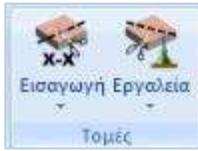
A prerequisite for the solution and sizing of the plates is the introduction of the sections. From the "Plates" field select "**Insert sections**" by **X** and/or **Z** and enter the sections by left-clicking. The direction of the section defines the direction of the main reinforcement.
