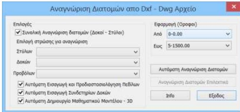
It is an automation system that recognizes beams, columns of any cross-section (T, P, C), plates and cantilevers, pedestals and connecting beams, while at the same time it automatically creates the mathematical model of the structure.
