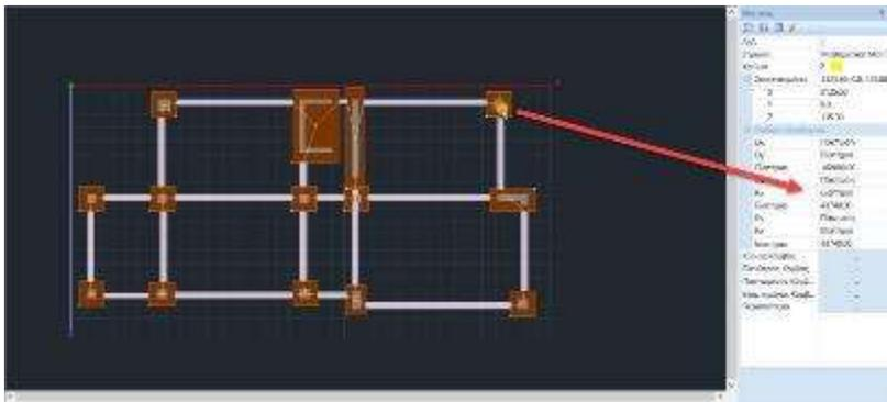
⚠ For the sake of completeness, the example also shows the manual way of inserting pedestals and connecting beams.
