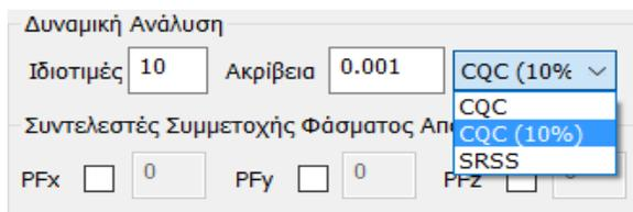
It is also possible to choose the mode of overlap of the eigenmodal responses either according to the Full Quadratic Parallelism CQC and CQC(10%) rule (3.6 EAK), or the Simple Quadratic Parallelism SRSS rule. Also, the results of the seismic action now include the results of the eigenmode analysis for the static scenarios.
