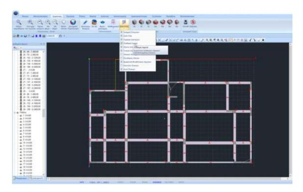
With the "Fixed Points" command in the "Tools" section you can modify the fixed point of the post and the fixed pass of the beam.
