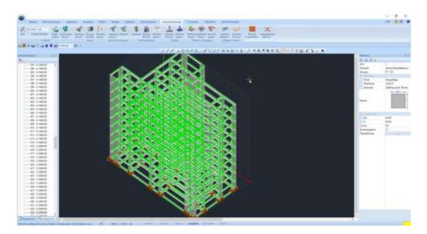
The aim in each study is to ensure that all data are adequate for all the controls required by the regulation. This example shows adequacy in both beams, columns and walls, as well as slabs.
